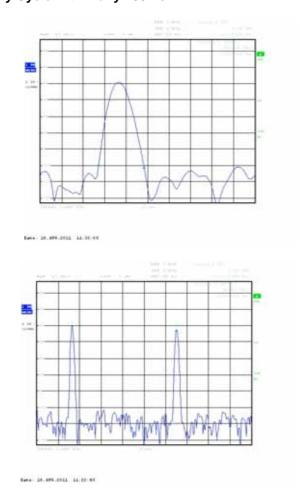
Every 29.19ms one impulse of 2.11ms was measured. Therefore, 3 impulses occur in any 100ms period.
