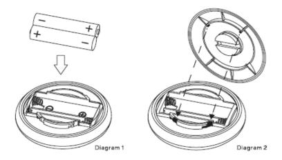
Once in place, insert the plastic key in the cover's slot and do a 10 degree twist clockwise to lock shut. To open, always use the key and make a 10 degree turn counterclockwise before replacing the batteries - using other tools such as coins may damage the surface of the remote (see Diagram 3).
