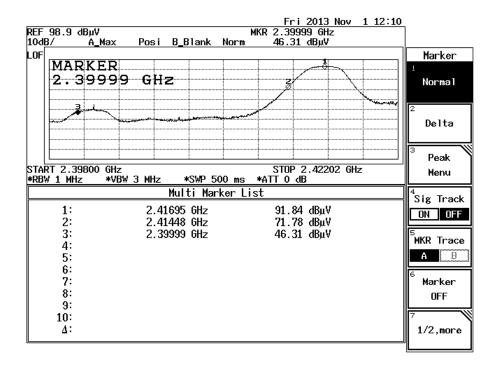
According to the page 12 of this report, the emission of the fundamental frequency 2417.0MHz is 91.82dBuV/m and 91.5dBuV/m for peak and average level respectively. Based on the delta method, the emission at the bandedge, 2400MHz, is more than 40dB below the fundamental and 20dB bandwidth falls in assigned band. It
