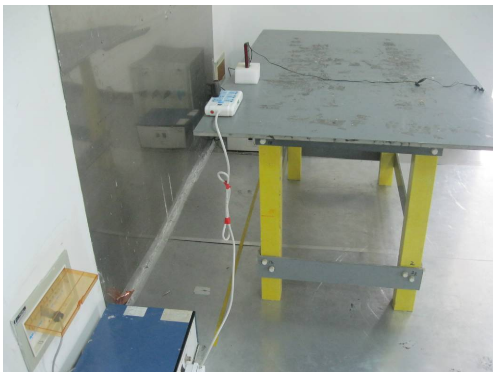
Conducted Emissions Test Setup Side View
