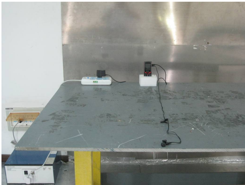
Conducted Emissions Test Setup Front View
