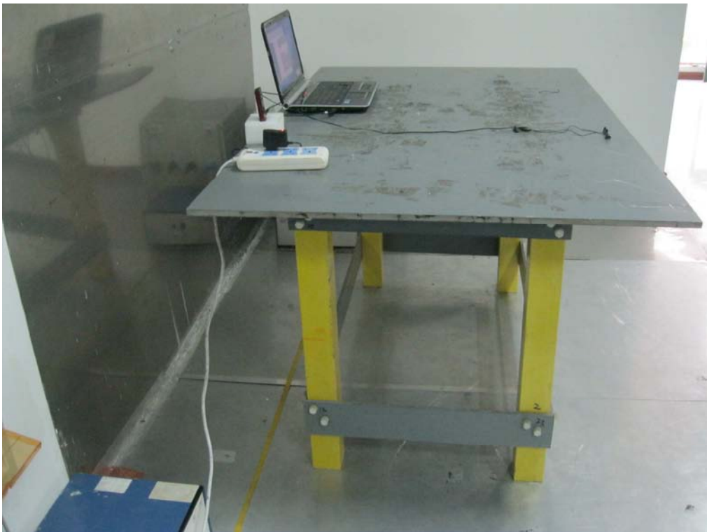
Conducted Emissions Test Setup Side View
