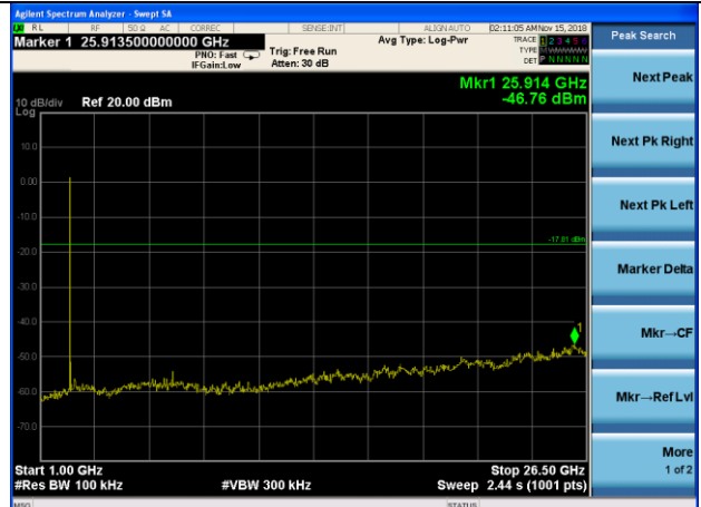
8-DPSK on channel 00
