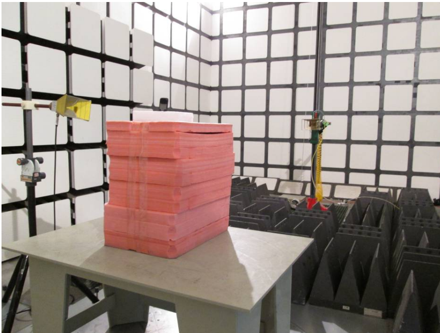
Radiated Emissions Test View (Above 1 GHz)
