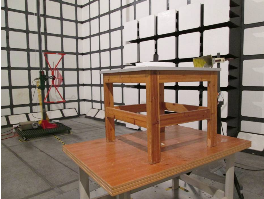
Radiated Emissions Test View (Below 1 GHz)
