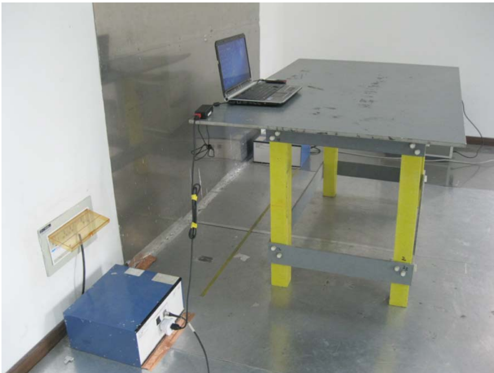
Conducted Emissions Test Setup - Side View
