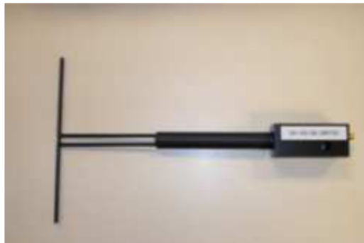
Figure 1 – Satimo COMOSAR Validation Dipole
