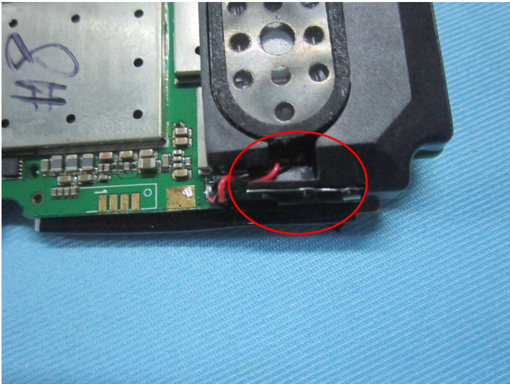
WIFI Antenna View
