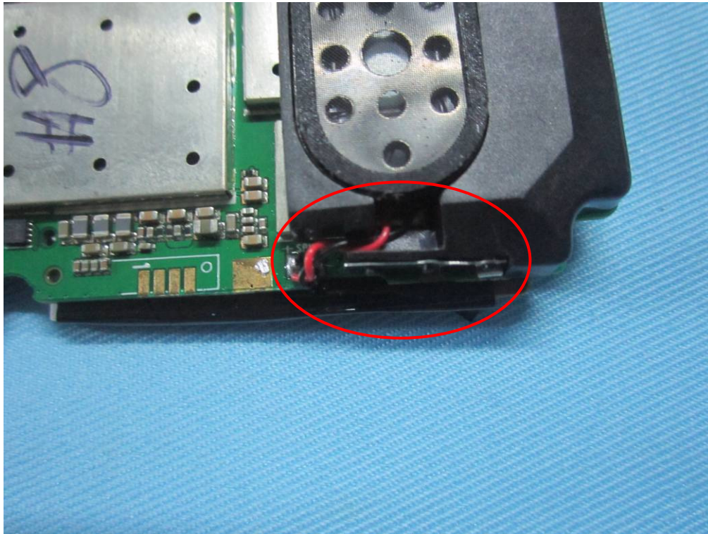
WIFI Antenna View
