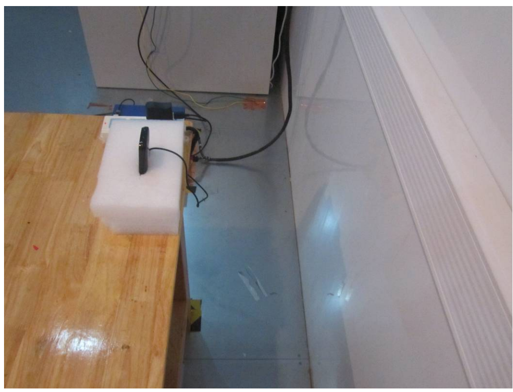
Conducted Emissions Test Setup Side View
