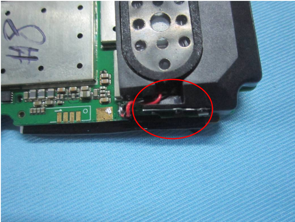
WIFI Antenna View
