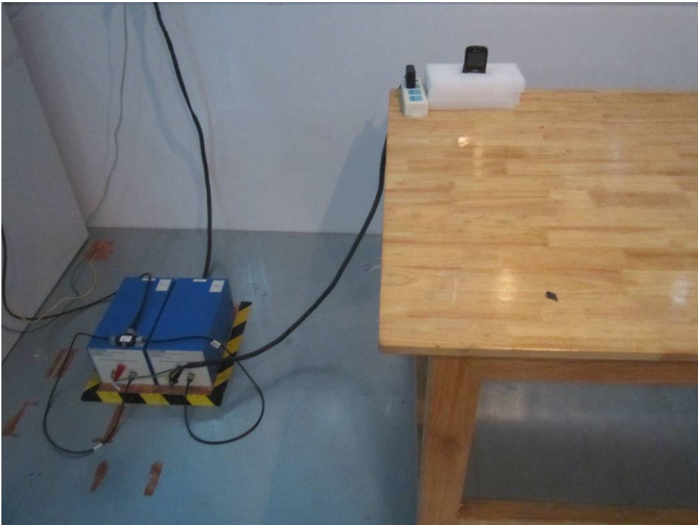
Conducted Emissions Test Setup Front View
