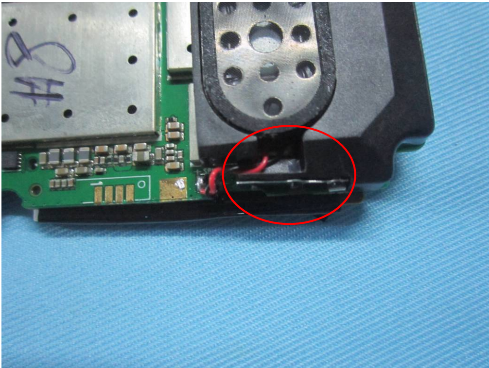
WIFI Antenna View
