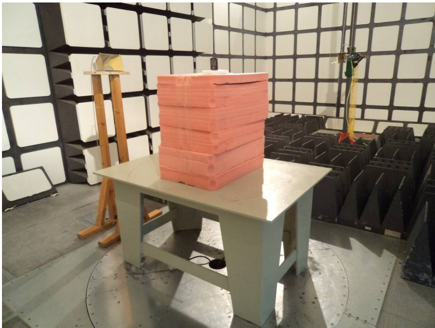
Radiated Emissions Test View (Above 1 GHz)
