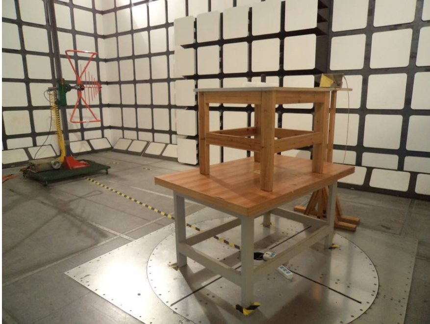
Radiated Emissions Test View (Below 1 GHz)
