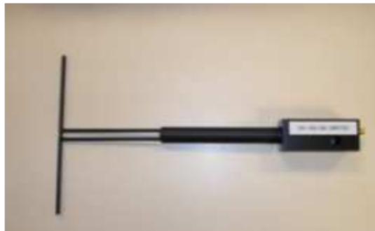
Figure 1 – Satimo COMOSAR Validation Dipole
