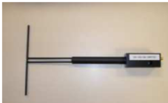
Figure 1 – Satimo COMOSAR Validation Dipole
