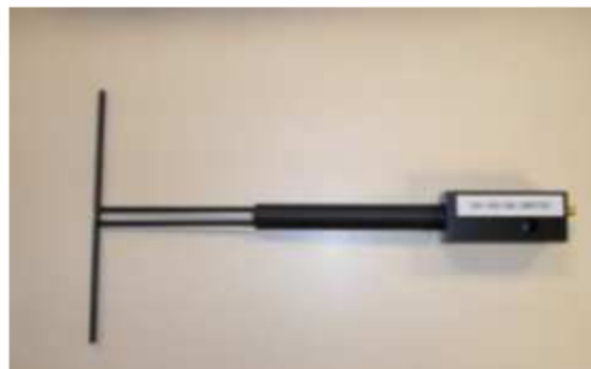
Figure 1 – Satimo COMOSAR Validation Dipole
