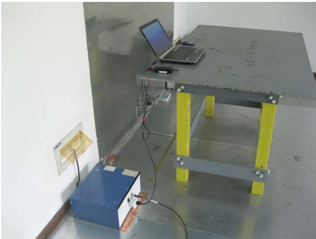
Conducted Emissions Test Setup - Side View
