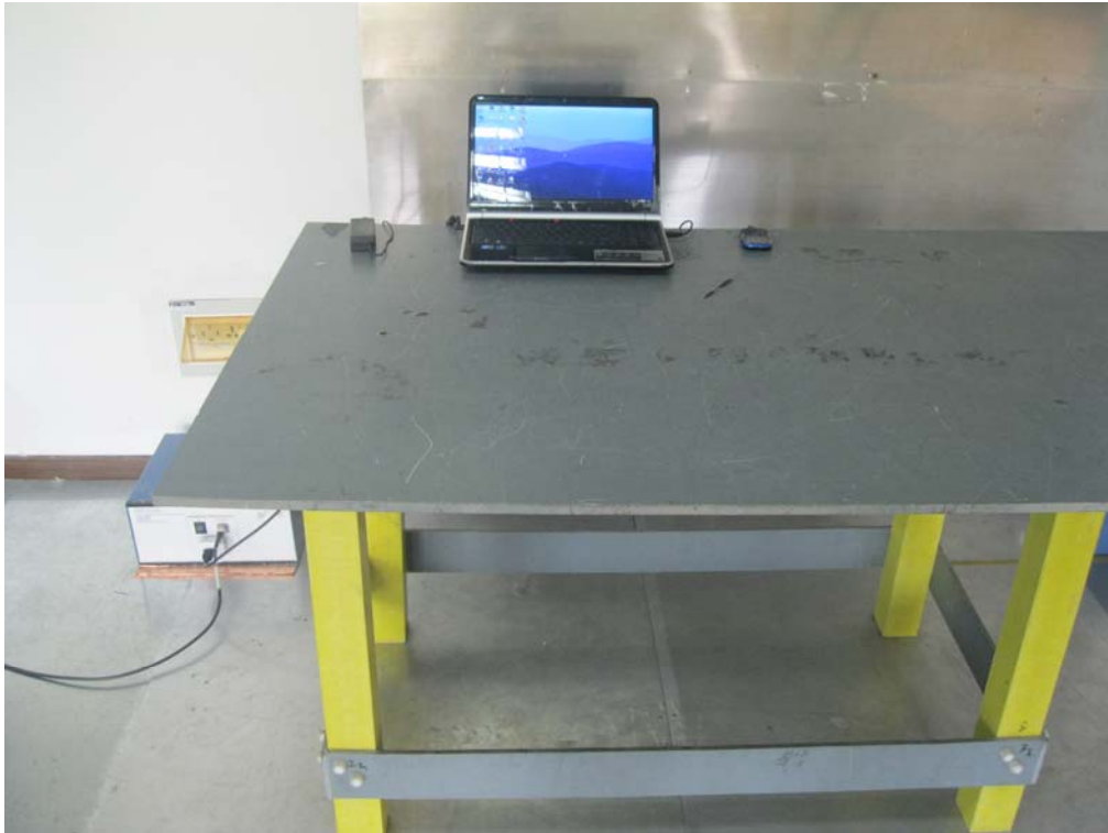
Conducted Emissions Test Setup - Front View
