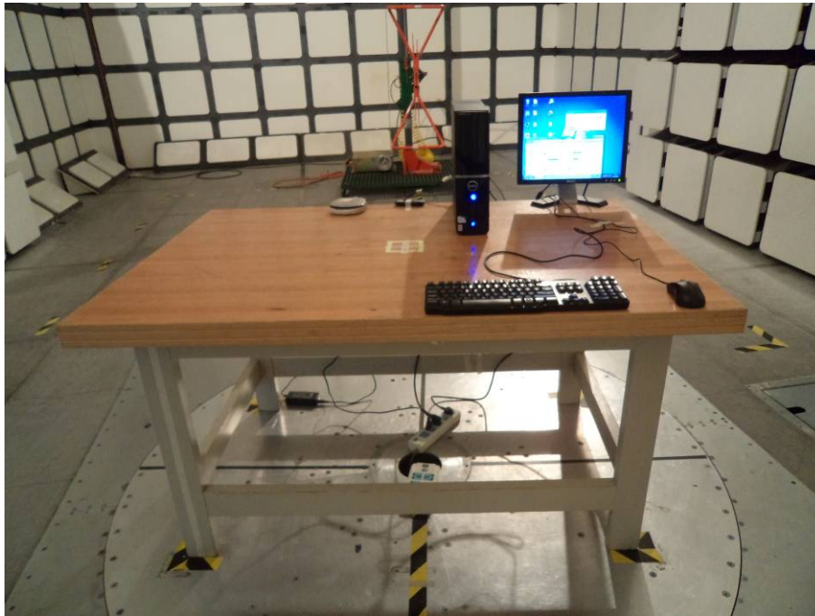
Radiated Emissions-Front View (Downlodging mode)
