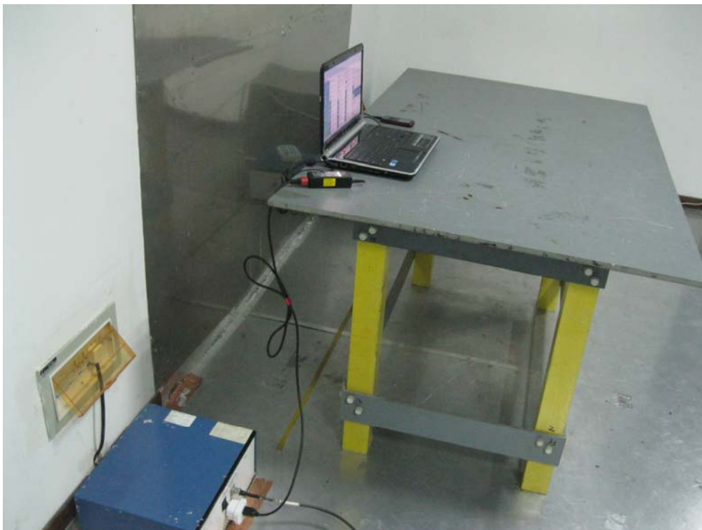
Conducted Emissions Test Setup - Side View
