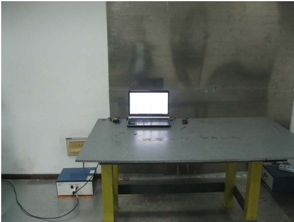
Conducted Emissions Test Setup - Front View
