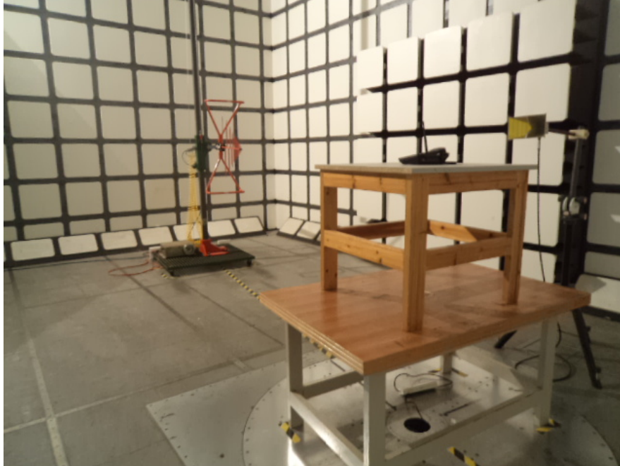
Radiated Emissions Test View (Below 1 GHz)
