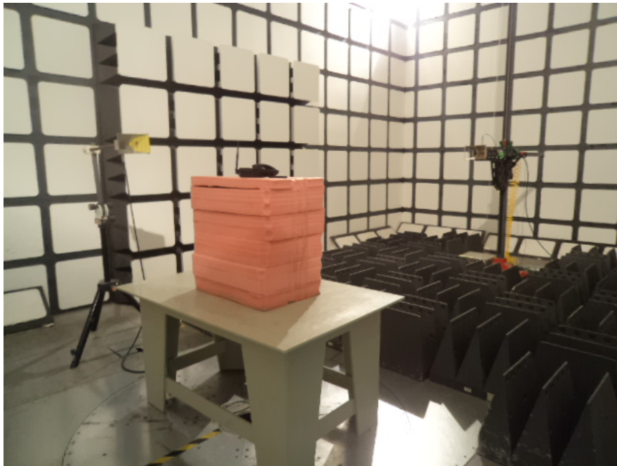
Radiated Emissions Test View (Above 1 GHz)
