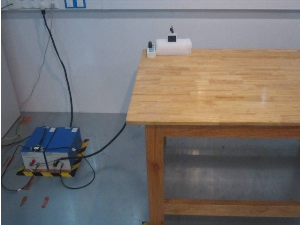
Conducted Emissions Test Setup Front View
