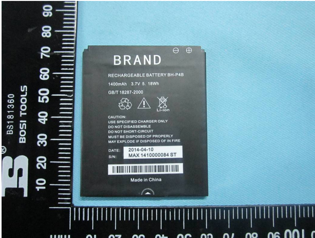
Battery - Top View
