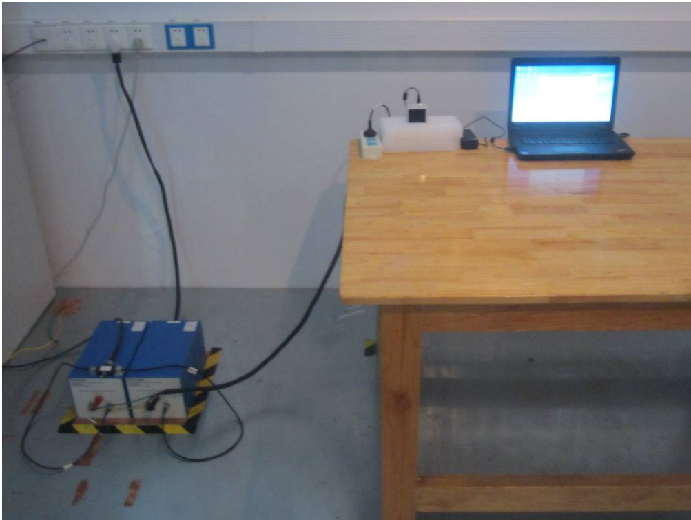
Conducted Emissions Test Setup Front View
