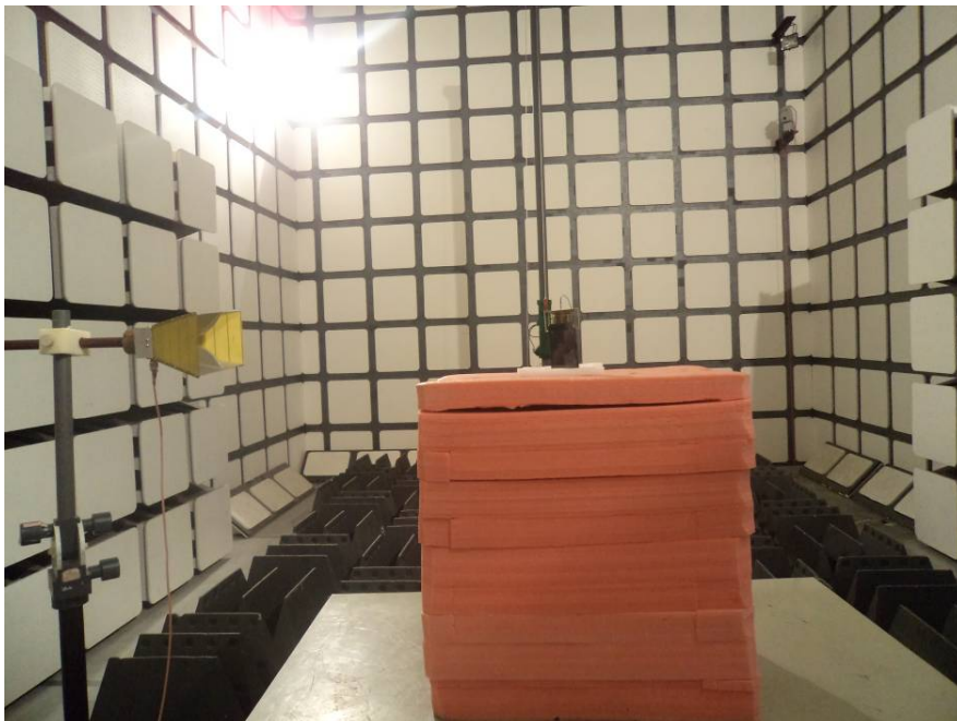
Radiated Emissions Test View (Above 1 GHz)
