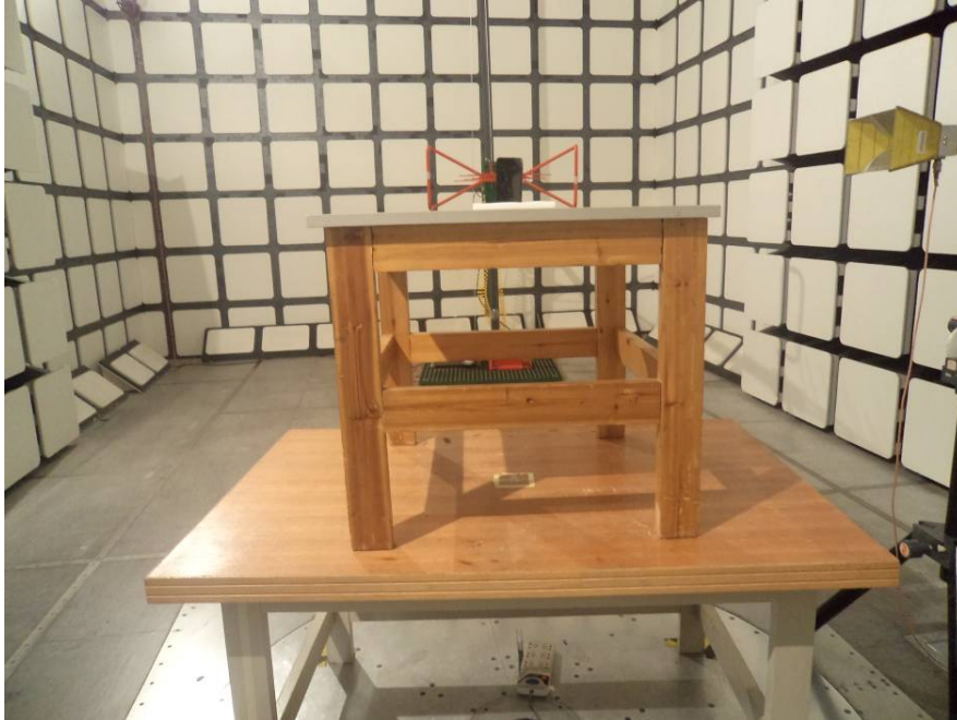
Radiated Emissions Test View (Below 1 GHz)
