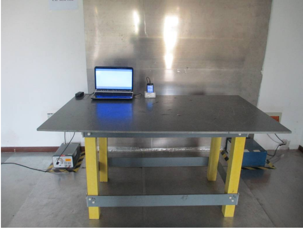
Conducted Emissions Test Setup Front View
