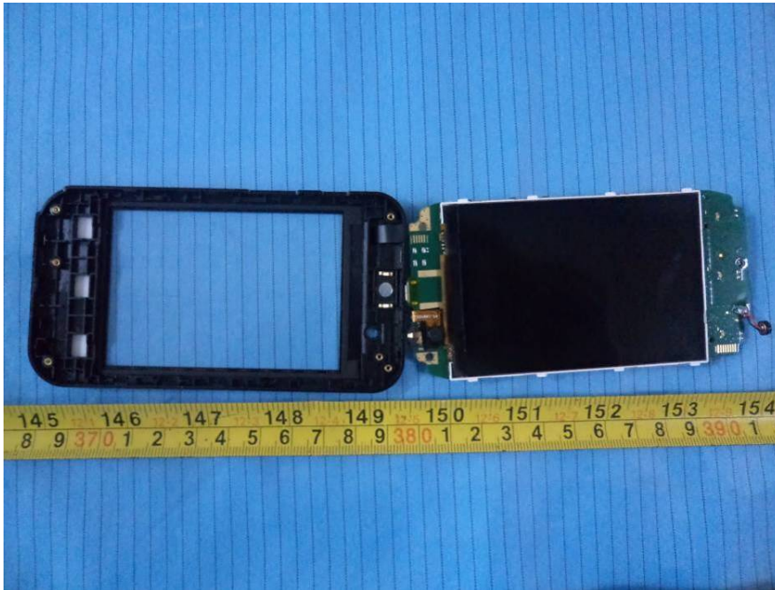
EUT – Cover off View 2
