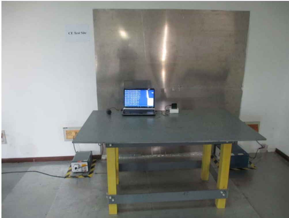
Conducted Emissions Test Setup Front View
