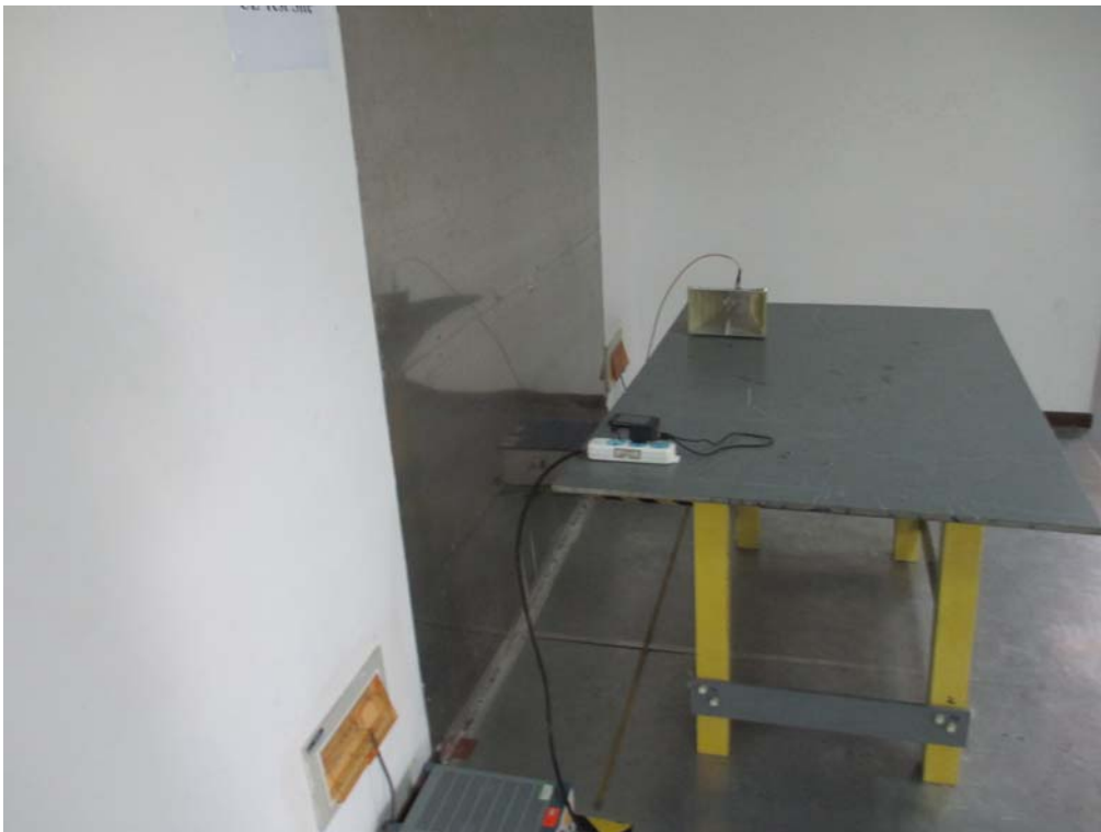
Conducted Emissions Test Setup Side View
