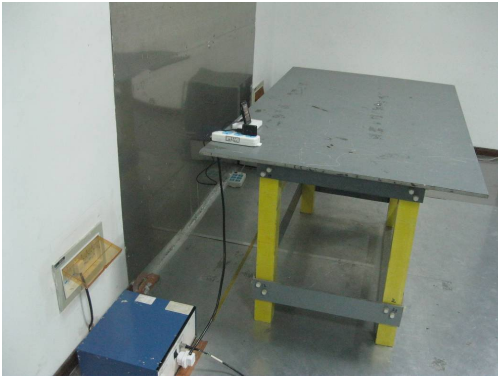
Conducted Emissions Test Setup (GPS receiving) - Side View
