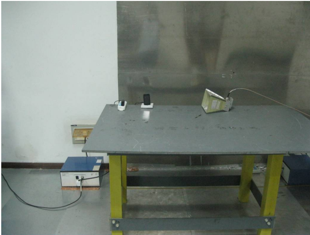
Conducted Emissions Test Setup - Front View
