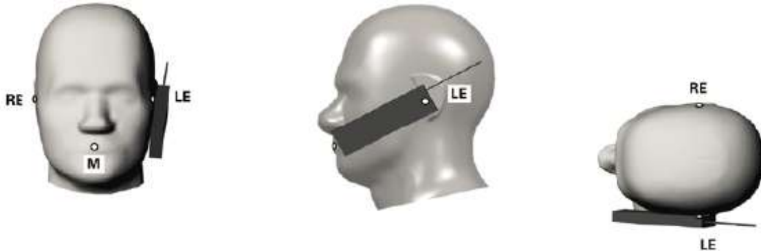
Fig. 11.3 Illustration for Cheek Position
