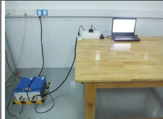
Conducted Emissions Test Setup – Front View
