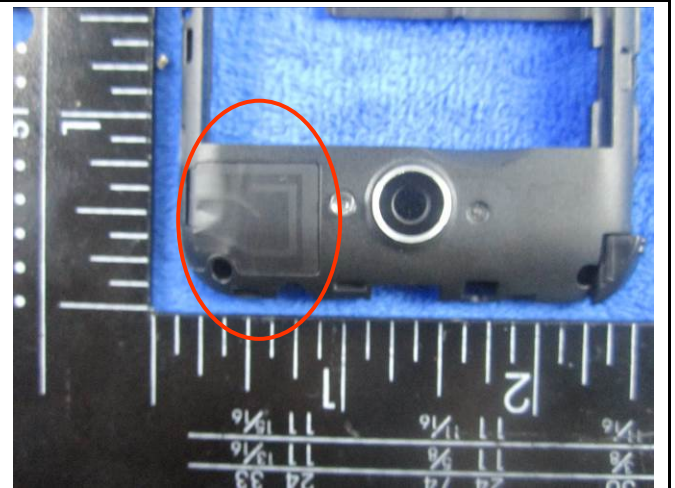
BT/WIFI Antenna View
