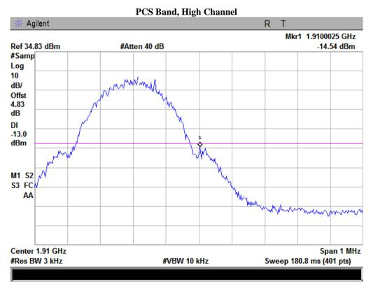
Note: Offset=Cable loss  $(4.5) + 10\log (3.24/3) = 4.5 + 0.33 = 4.83 \text{ dB}$
