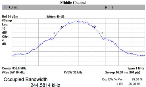
Transmit Freq Error -3.242 kHz x dB Bandwidth 315.186 kHz\*
