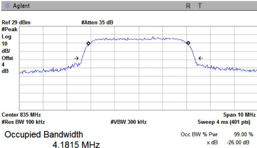
Transmit Freq Error -5.792 kHz x dB Bandwidth 4.718 MHz
