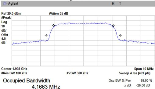
Transmit Freq Error 8.251 kHz x dB Bandwidth 4.710 MHz
