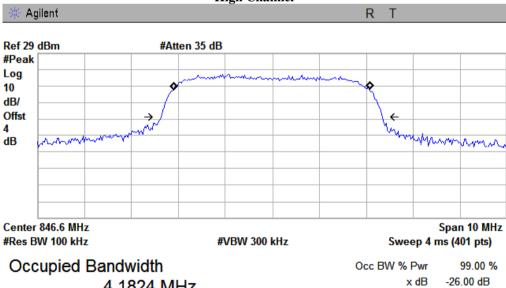
Transmit Freq Error -18.003 kHz x dB Bandwidth 4.708 MHz
