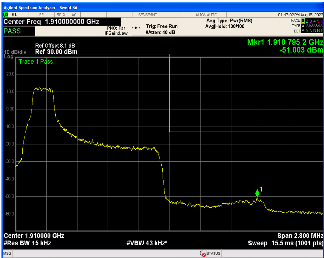
Band2 16QAM BW=1.4MHz Channel=19193 RB Size=1 Position=#Max
