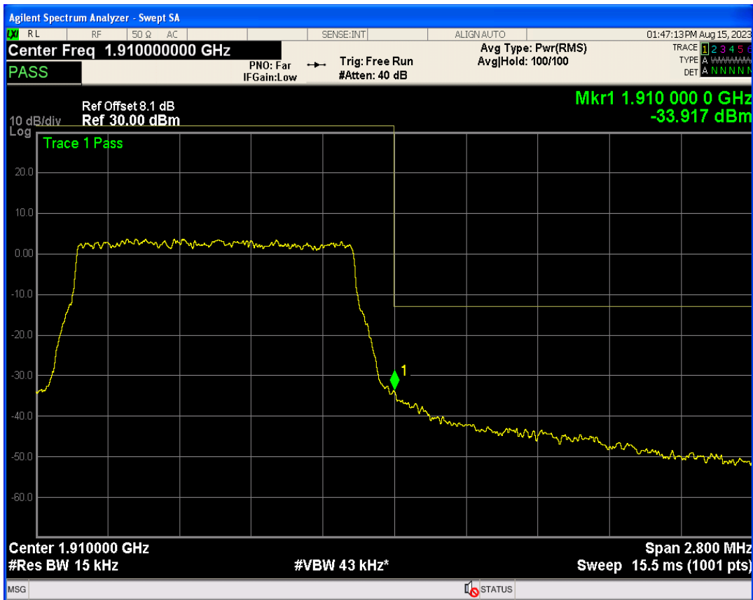
Band2 QPSK BW=3MHz Channel=18615 RB Size=1 Position=#0
