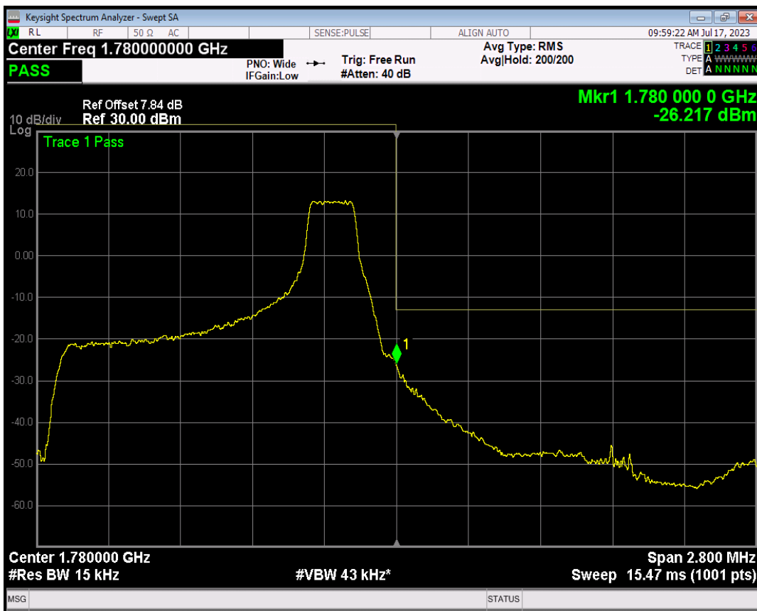
Band66 16QAM BW=1.4MHz Channel=132665 RB Size=6 Position=#0
