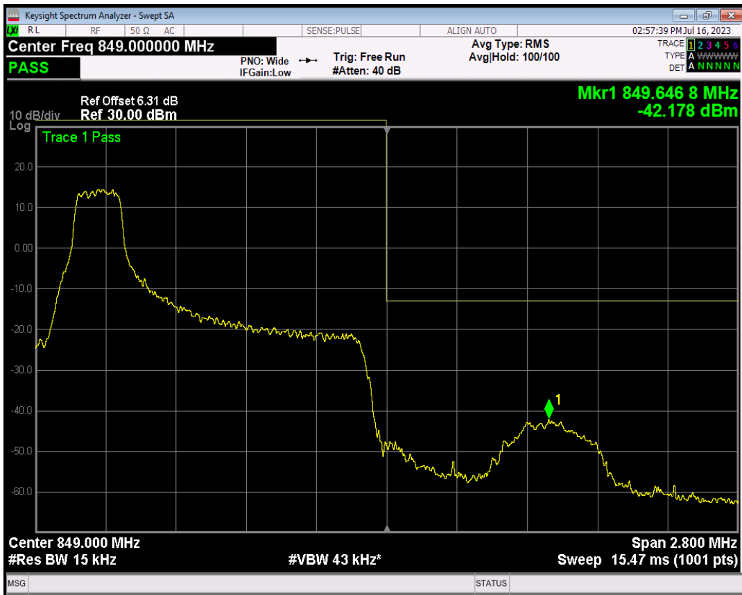
Band5 QPSK BW=1.4MHz Channel=20643 RB Size=1 Position=#Max
