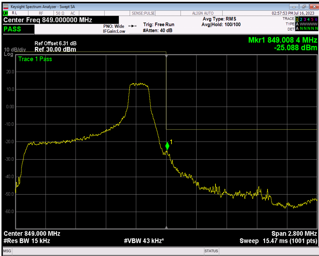
Band5 16QAM BW=1.4MHz Channel=20643 RB Size=6 Position=#0
