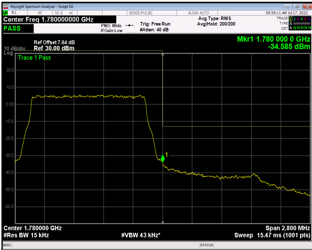
Band66 16QAM BW=1.4MHz Channel=132665 RB Size=1 Position=#0
