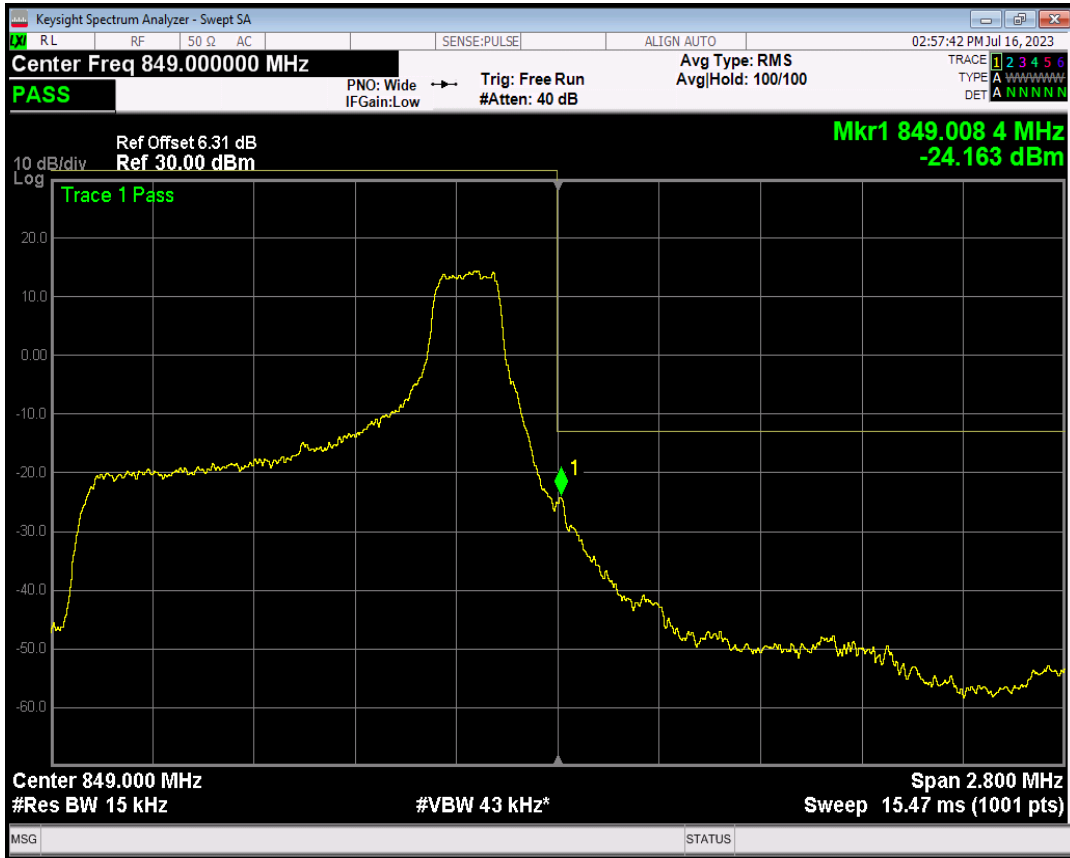
Band5 QPSK BW=1.4MHz Channel=20643 RB Size=6 Position=#0
