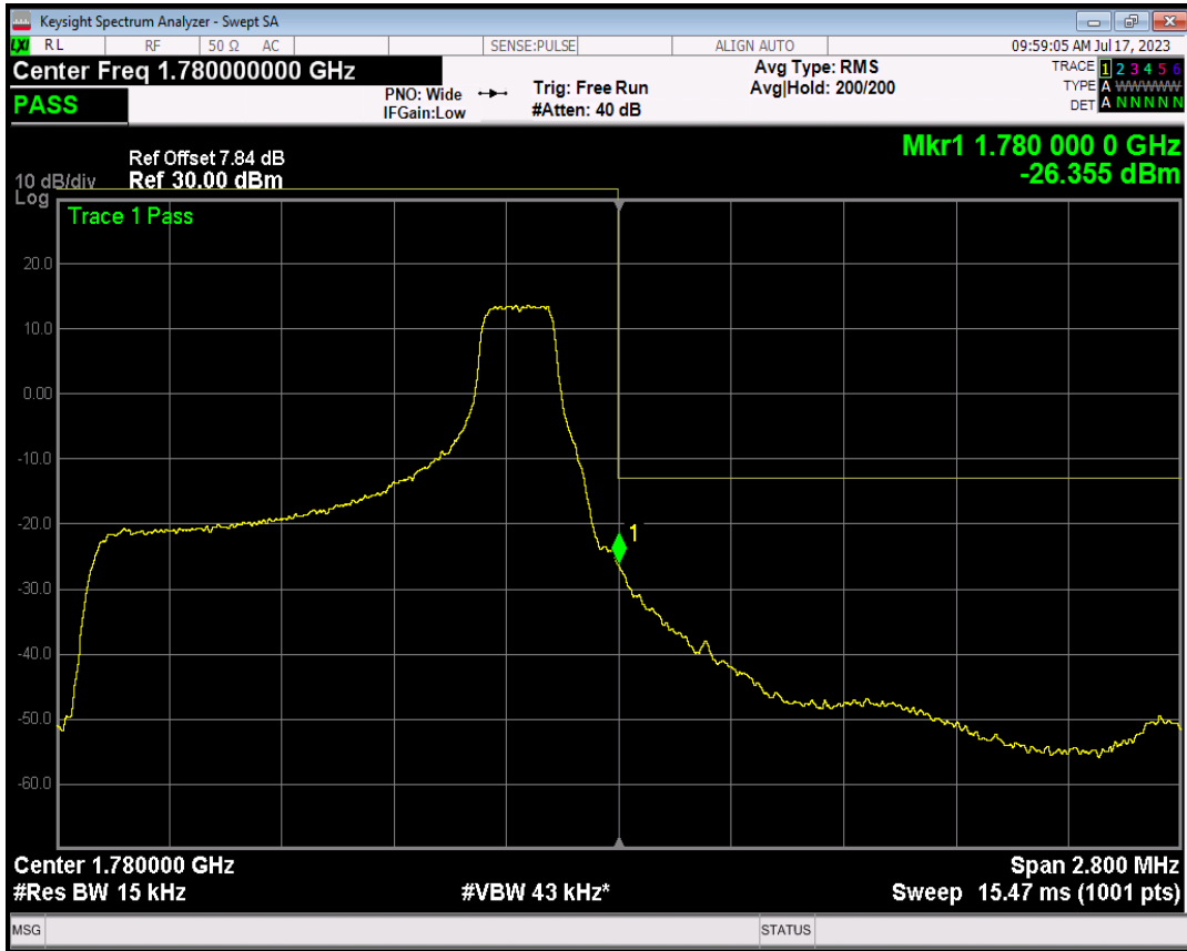
Band66 QPSK BW=1.4MHz Channel=132665 RB Size=6 Position=#0
