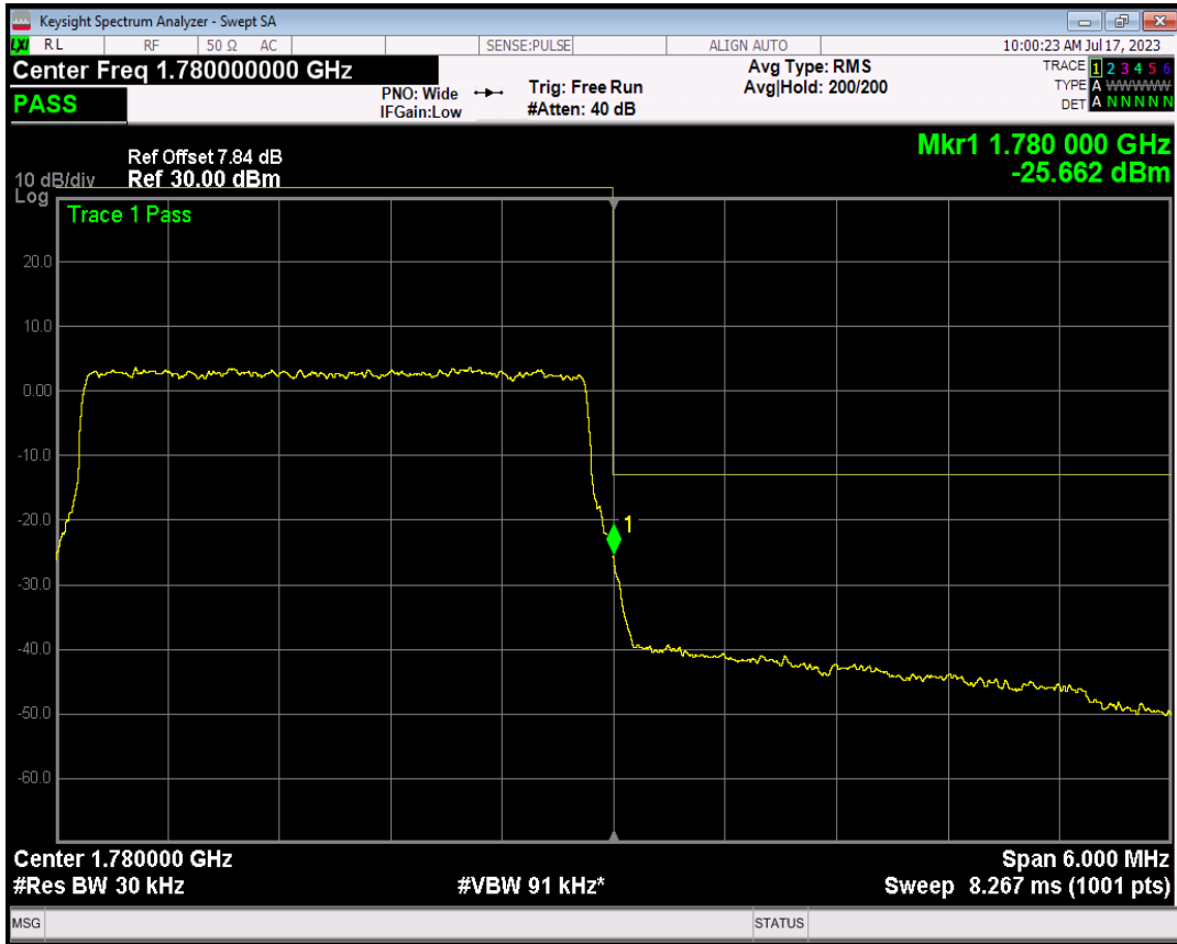
Band66 QPSK BW=5MHz Channel=131997 RB Size=1 Position=#0
