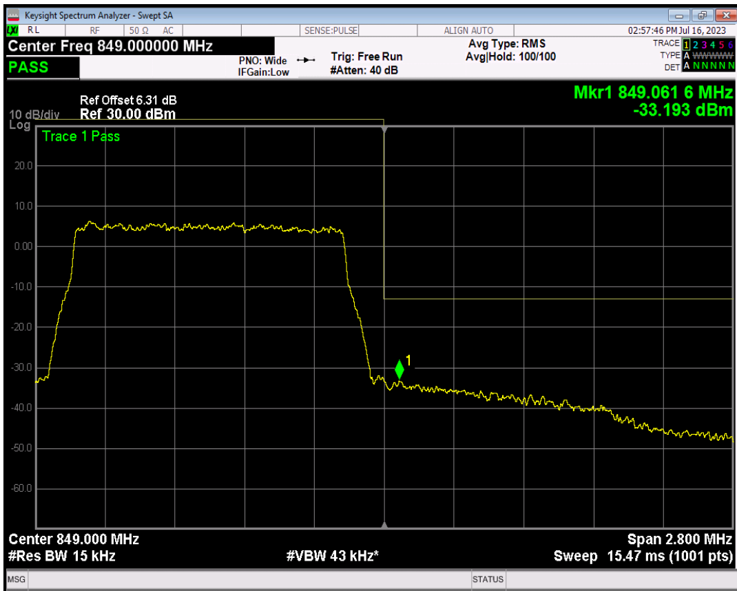
Band5 16QAM BW=1.4MHz Channel=20643 RB Size=1 Position=#0
