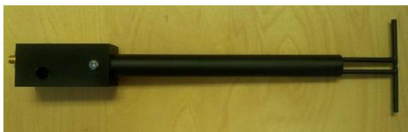
Figure 1 – MVG COMOSAR Validation Dipole
