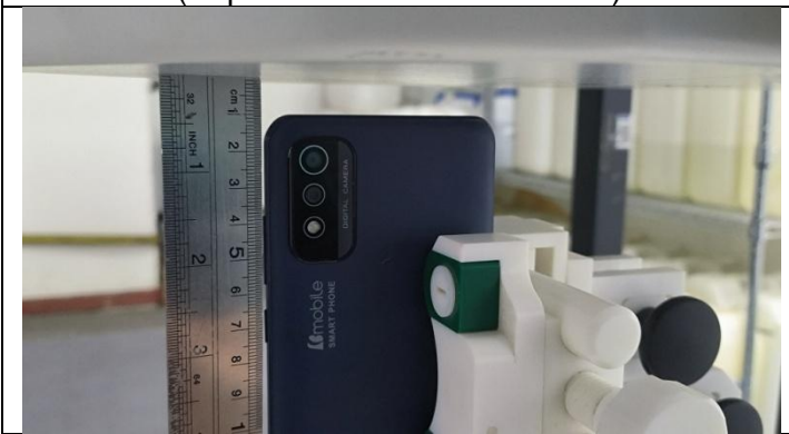
Top Side (Separation distance of 10mm)
