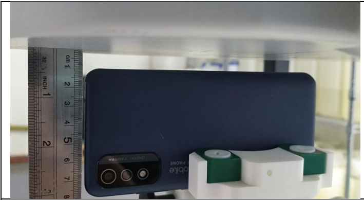
Top Side (Separation distance of 10mm)
