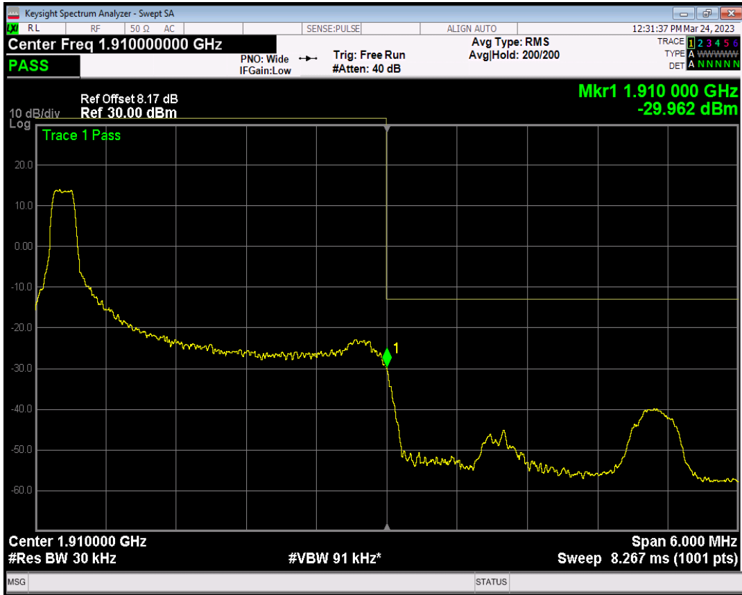
Band2 QAM16 BW=3MHz Channel=19185 RB Size=1 Position=#Max
