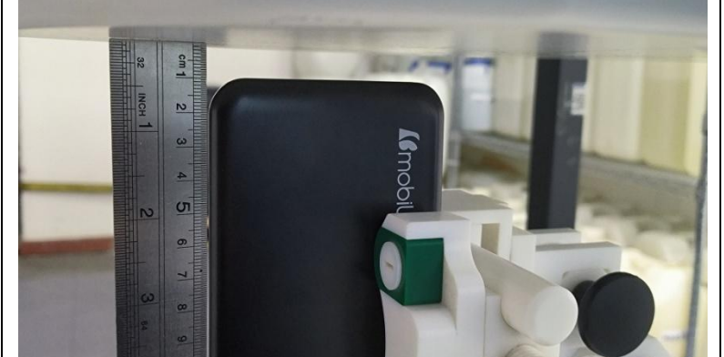
Bottom Side (Separation distance of 10mm)
