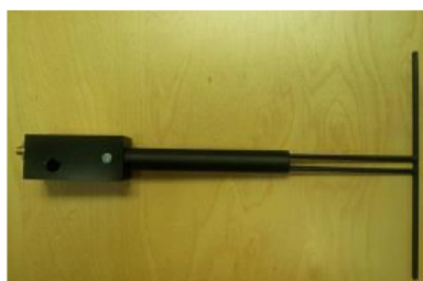
Figure 1 – MVG COMOSAR Validation Dipole
