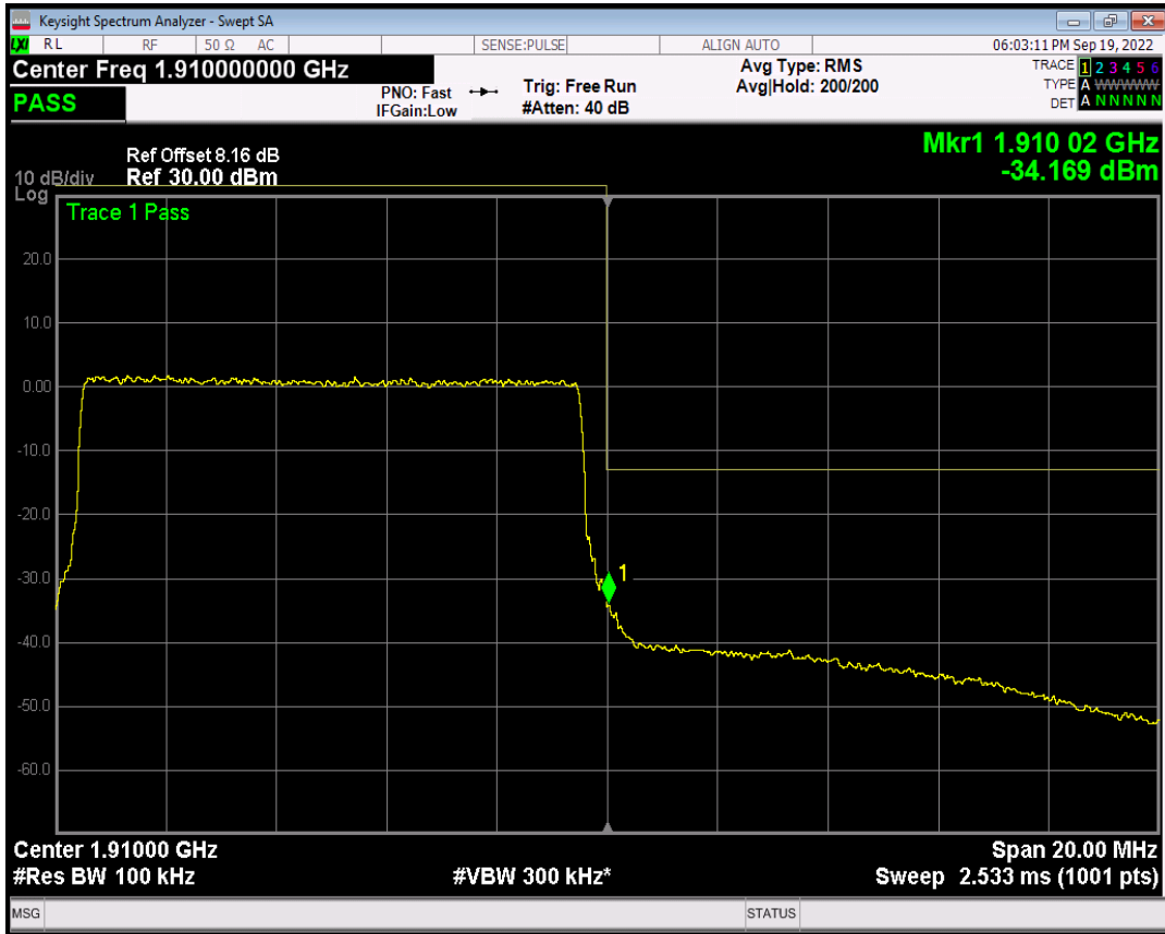
Band2 QAM16 BW=15MHz Channel=18675 RB Size=1 Position=#0
