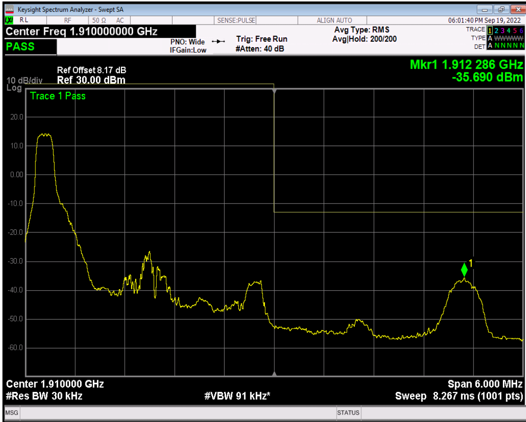
Band2 QAM16 BW=3MHz Channel=19185 RB Size=1 Position=#Max
