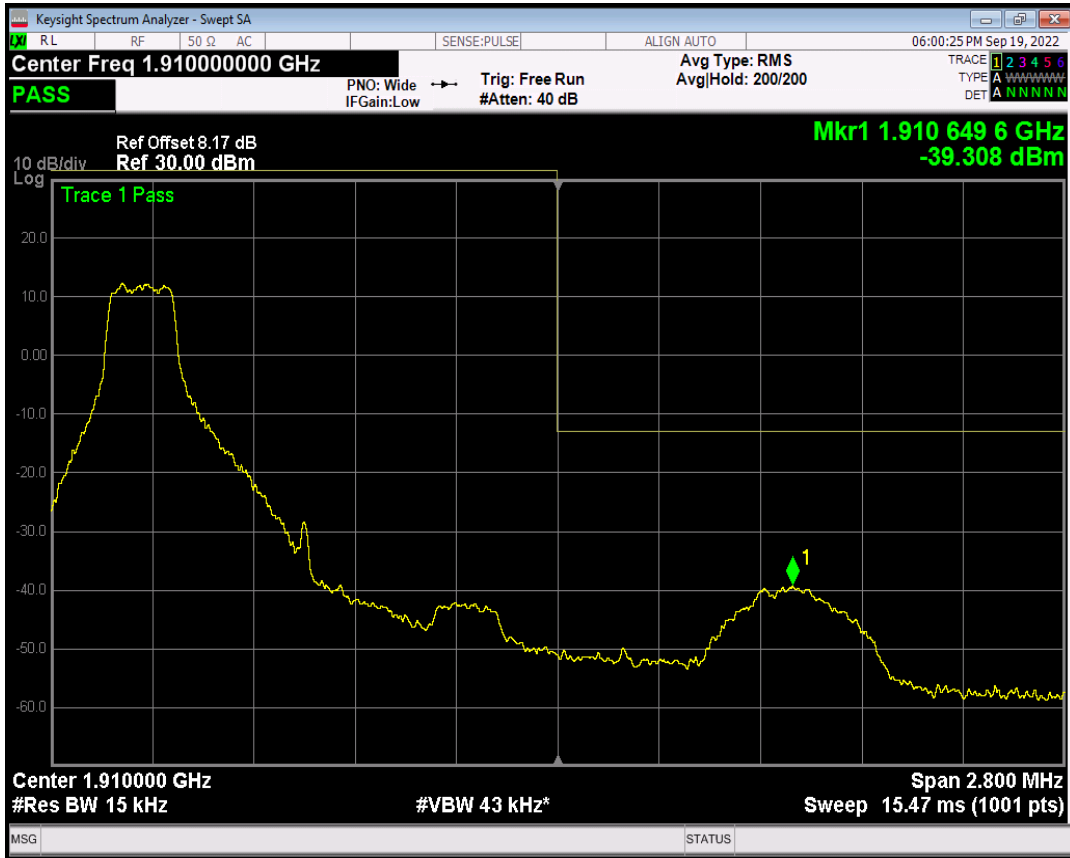
Band2 QPSK BW=1.4MHz Channel=19193 RB Size=1 Position=#Max
