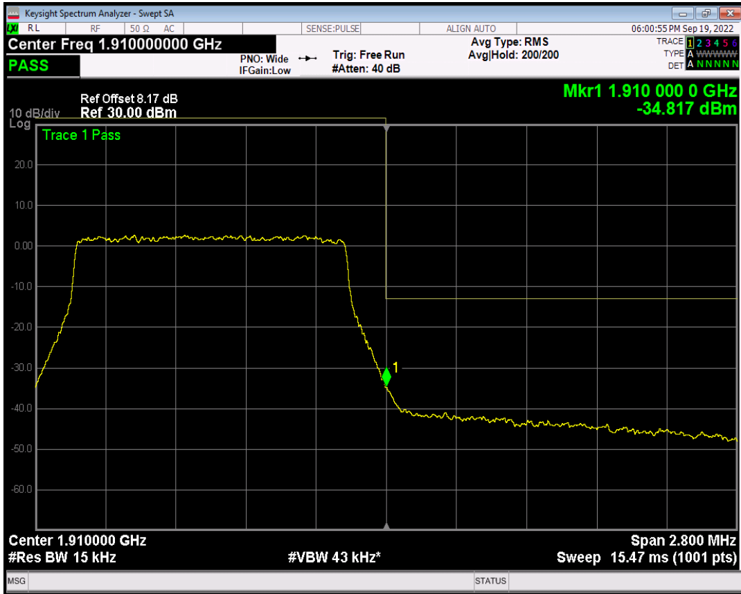
Band2 QAM16 BW=10MHz Channel=18650 RB Size=1 Position=#0
