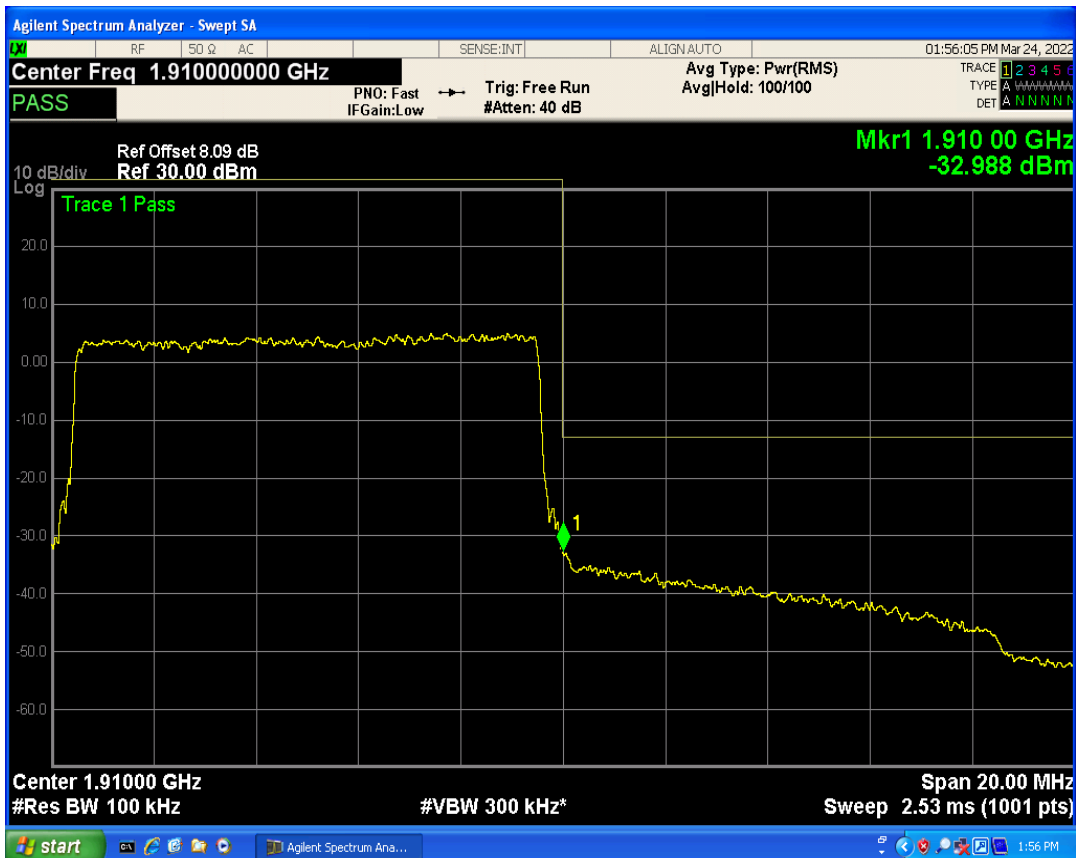
Band2 QAM16 BW=10MHz Channel=19150 RB Size=1 Position=#0
