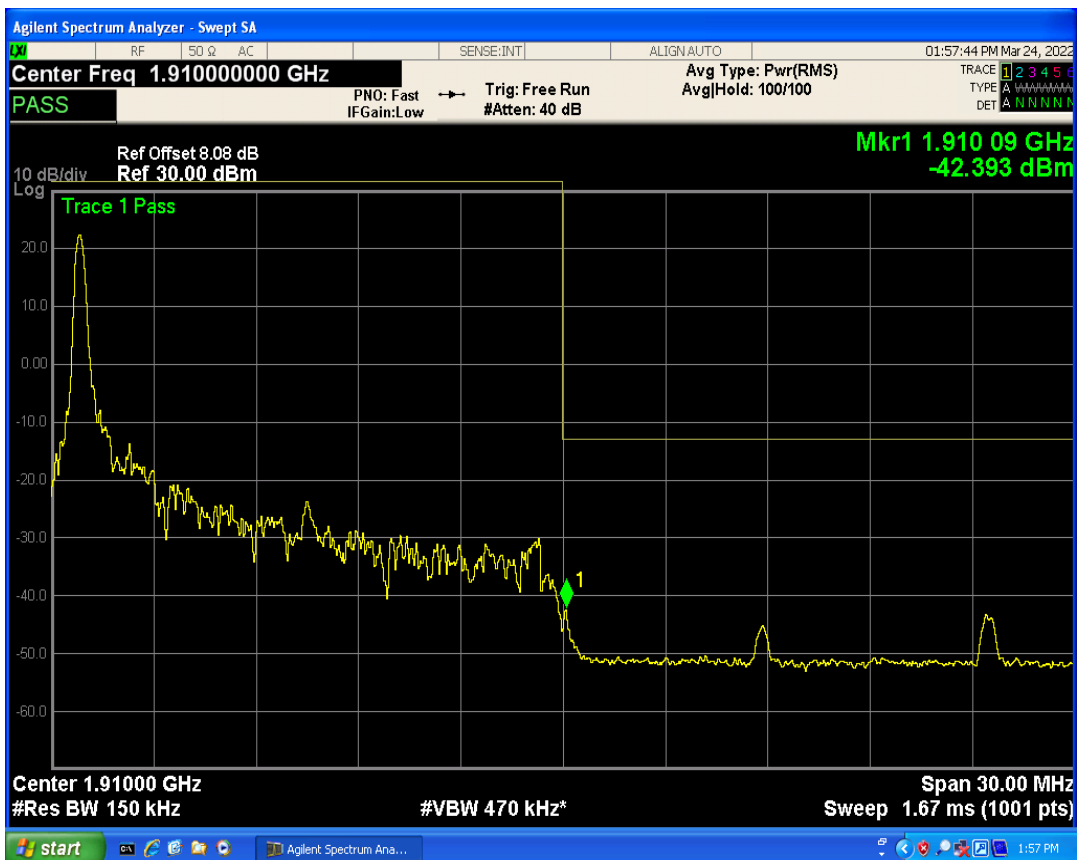
Band2 QPSK BW=15MHz Channel=19125 RB Size=1 Position=#Max
