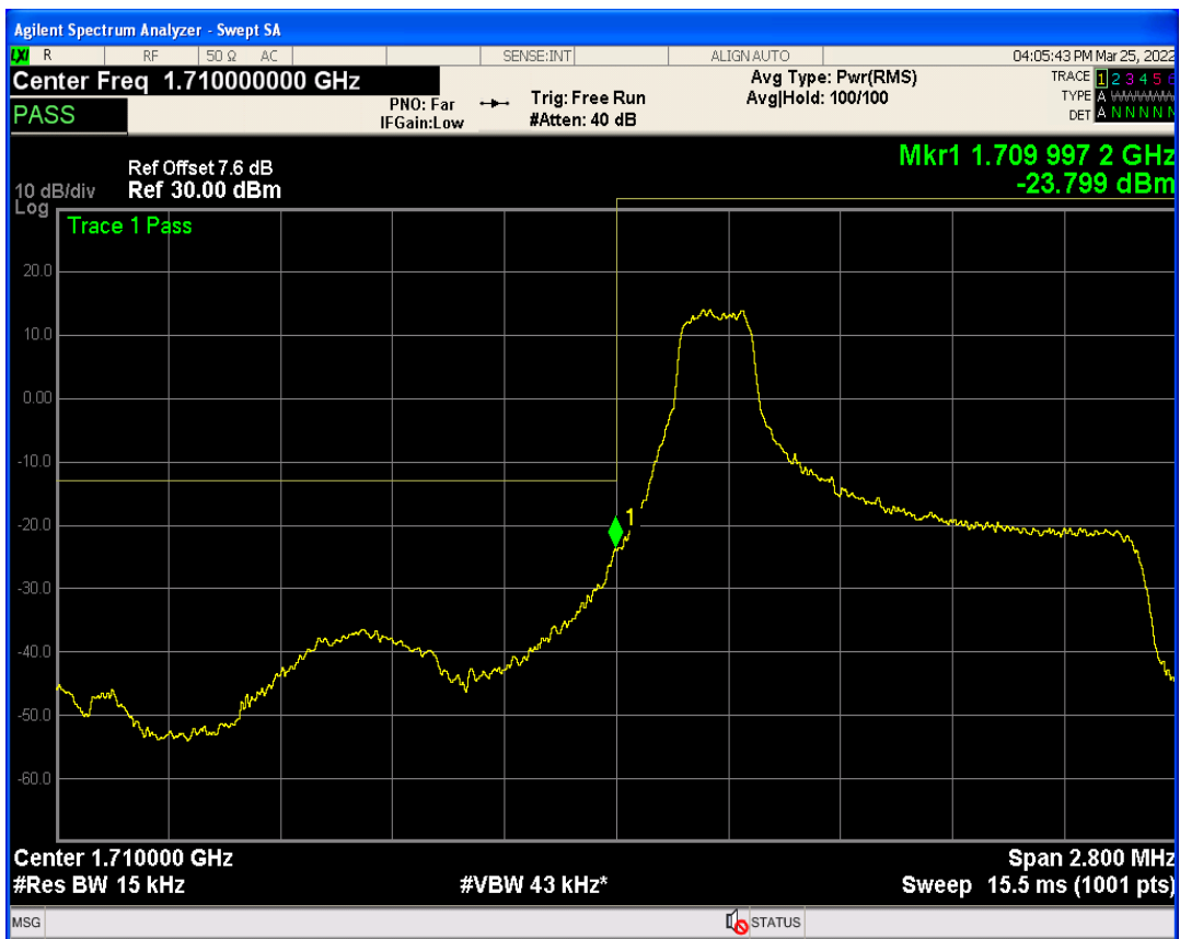
Band4 QPSK BW=1.4MHz Channel=19957 RB Size=1 Position=#Max
