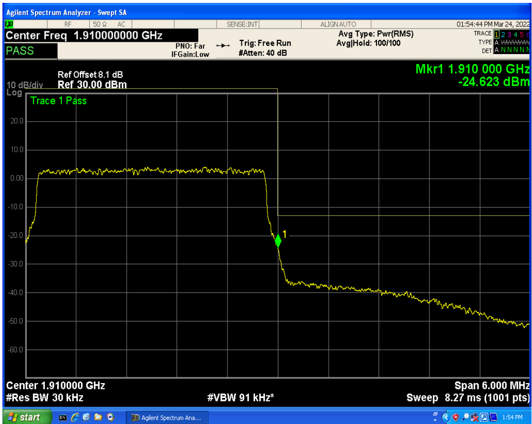
Band2 QPSK BW=5MHz Channel=18625 RB Size=1 Position=#Max
