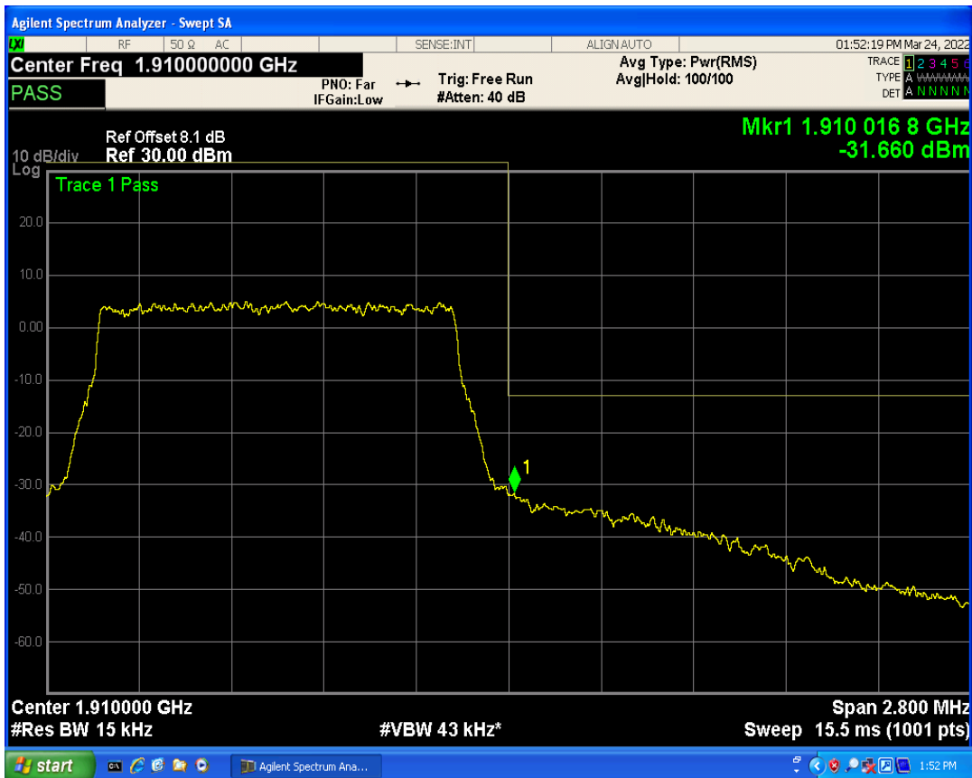
Band2 QAM16 BW=1.4MHz Channel=19193 RB Size=1 Position=#Max
