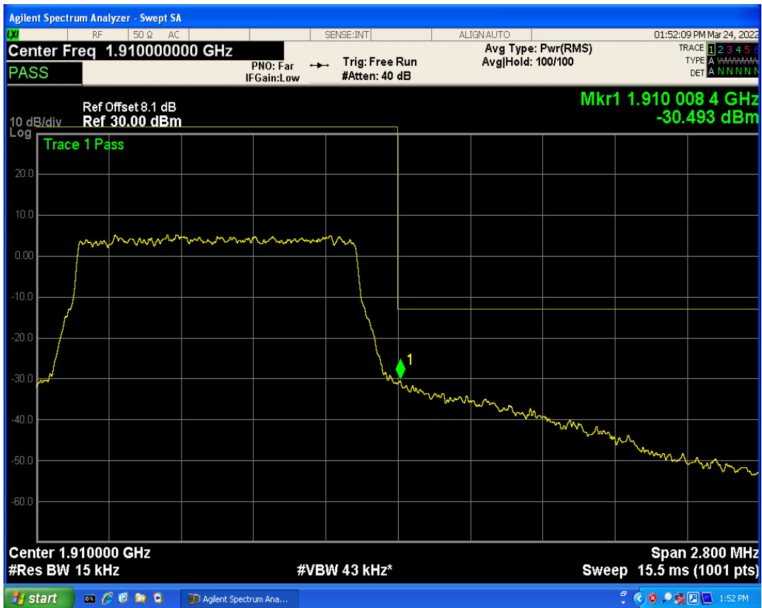
Band2 QPSK BW=1.4MHz Channel=19193 RB Size=1 Position=#Max
