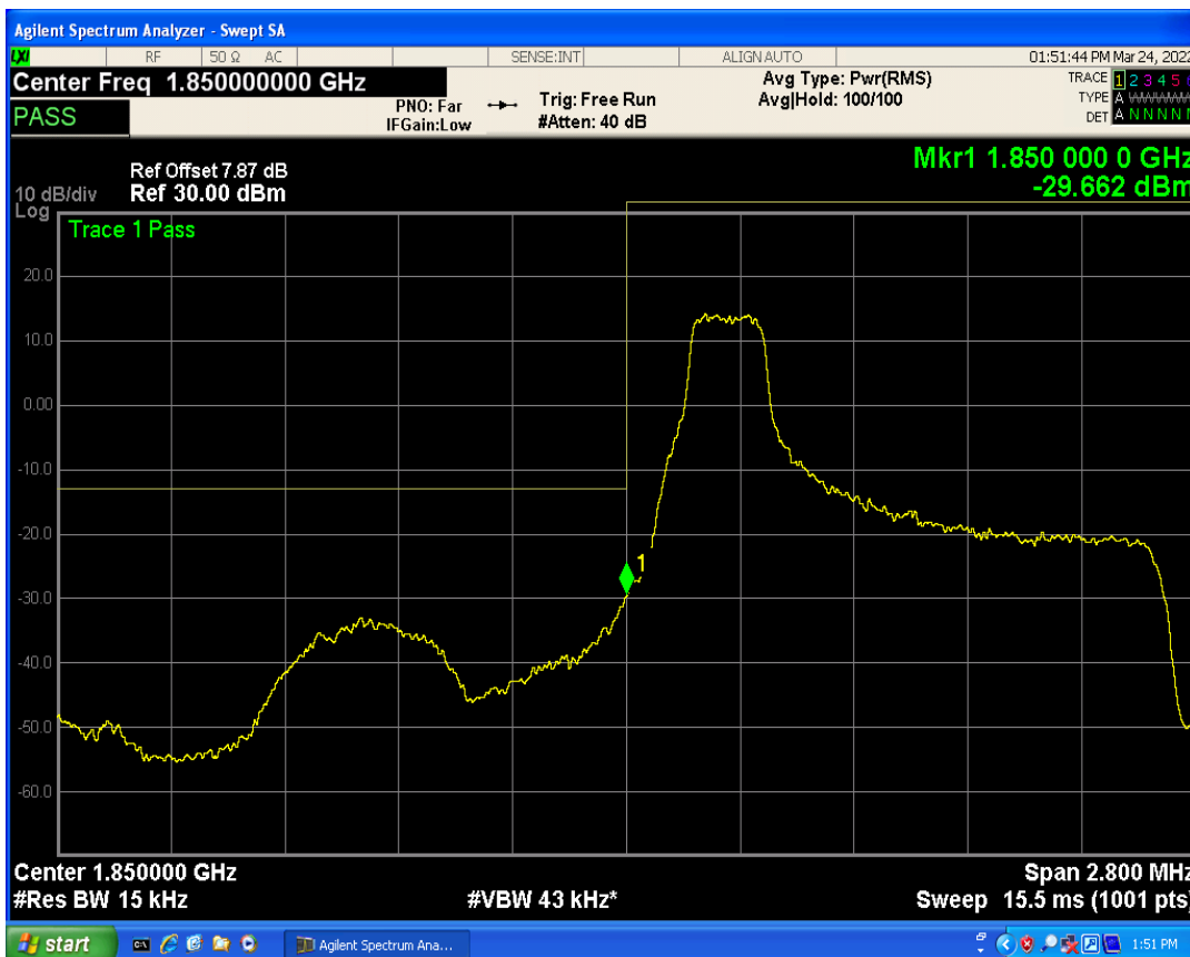
Band2 QPSK BW=1.4MHz Channel=18607 RB Size=1 Position=#0
