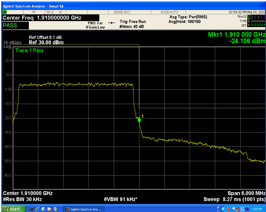
Band2 QAM16 BW=3MHz Channel=19185 RB Size=1 Position=#0
