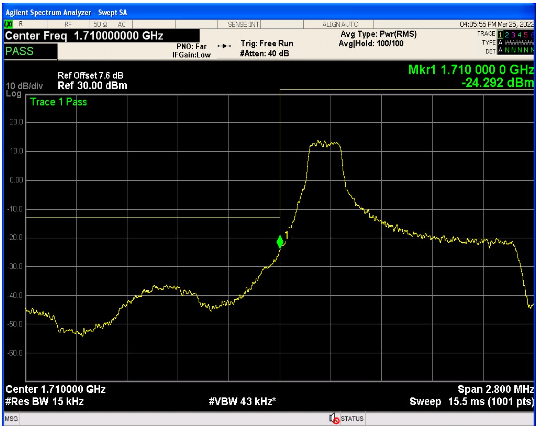
Band4 QPSK BW=1.4MHz Channel=19957 RB Size=6 Position=#0
