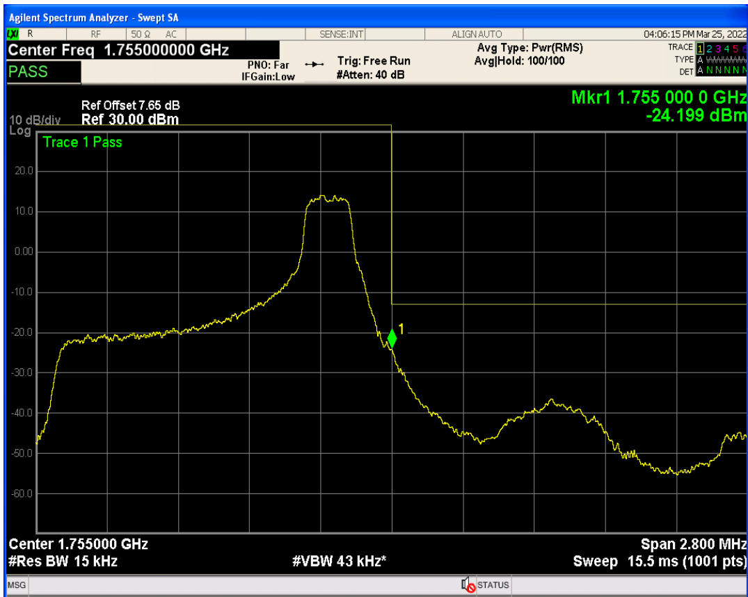
Band4 QPSK BW=1.4MHz Channel=20393 RB Size=6 Position=#0
