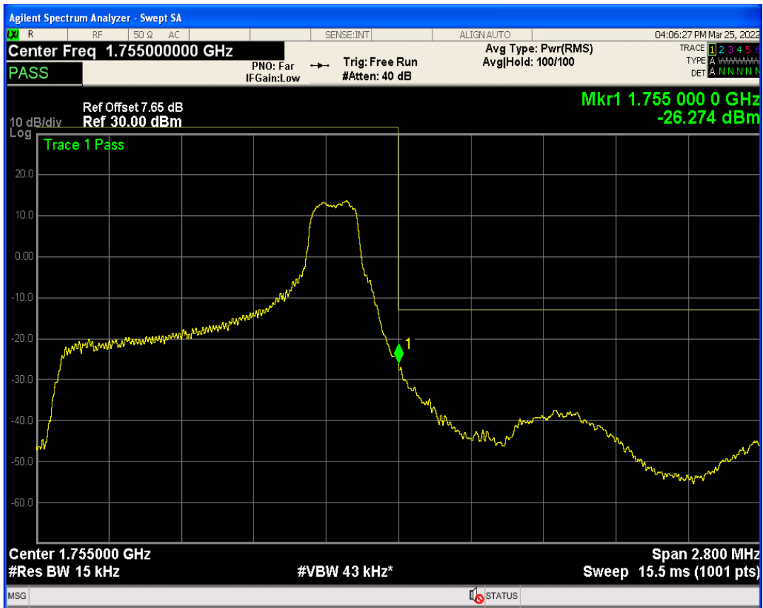
Band4 QPSK BW=3MHz Channel=19965 RB Size=1 Position=#Max
