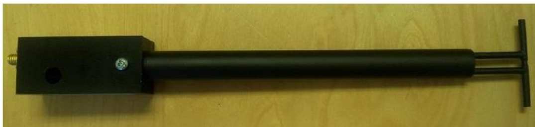
Figure 1 – MVG COMOSAR Validation Dipole
