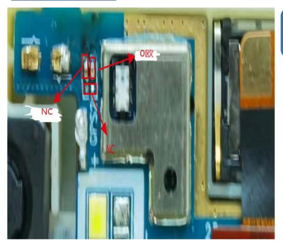
1. Parallel NC \_ Serial O ohms, as shown in the figure
