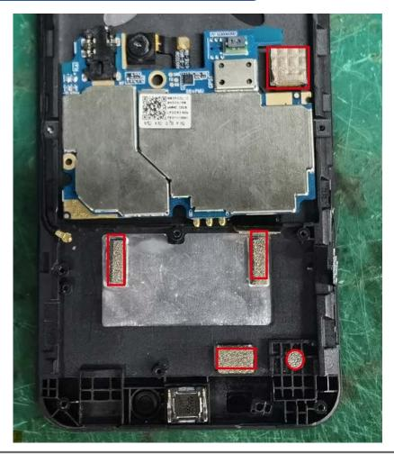
1. The motherboard and the screen are grounded, please increase the thickness of the sponge, all the trial production machines are not Connect to the ground, so the GPS will be very poor.
