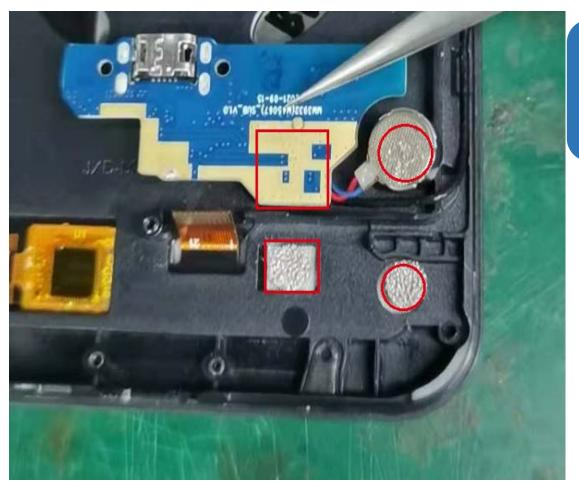
The small board is grounded, and the motor is grounded
