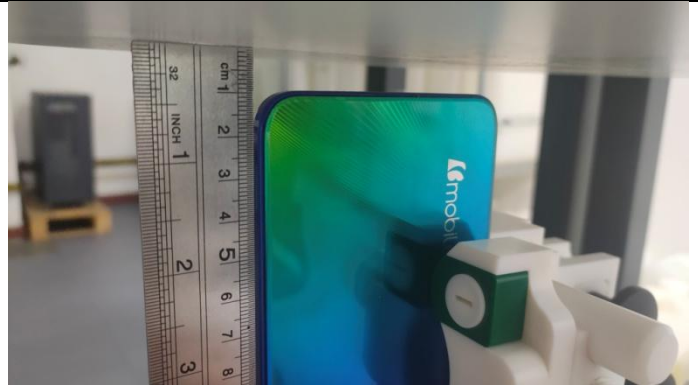
Bottom Side (Separation distance of 10mm)
