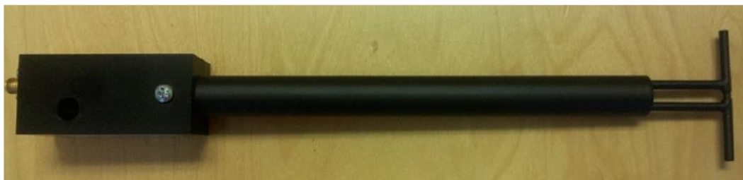
Figure 1 – MVG COMOSAR Validation Dipole
