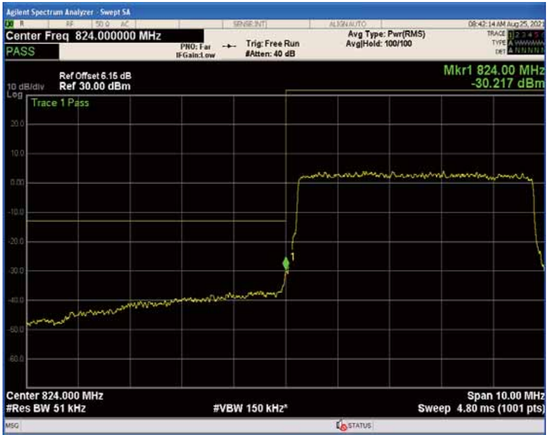
Band5 QPSK BW=5MHz Channel=20625 RB Size=1 Position=#0
