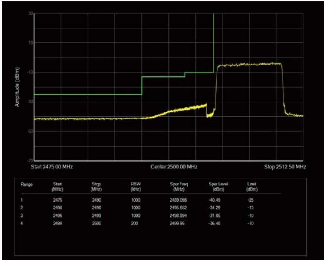
Band7 QPSK BW=10MHz Channel=20800 RB Size=1 Position=#Max
