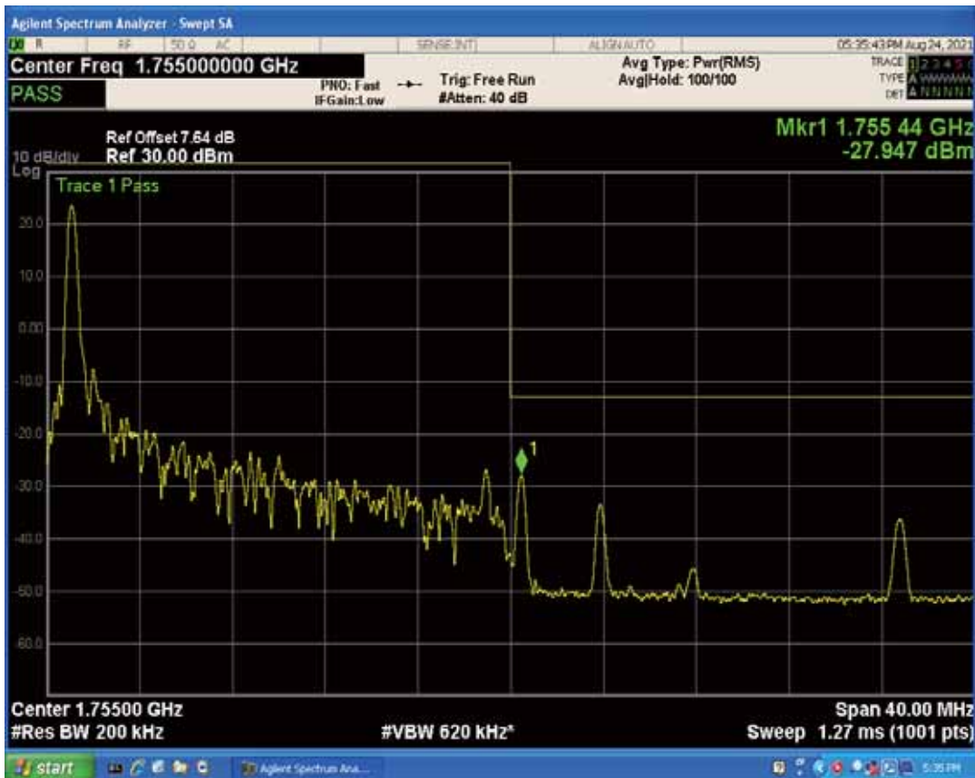
Band4 QPSK BW=20MHz Channel=20300 RB Size=1 Position=#Max
