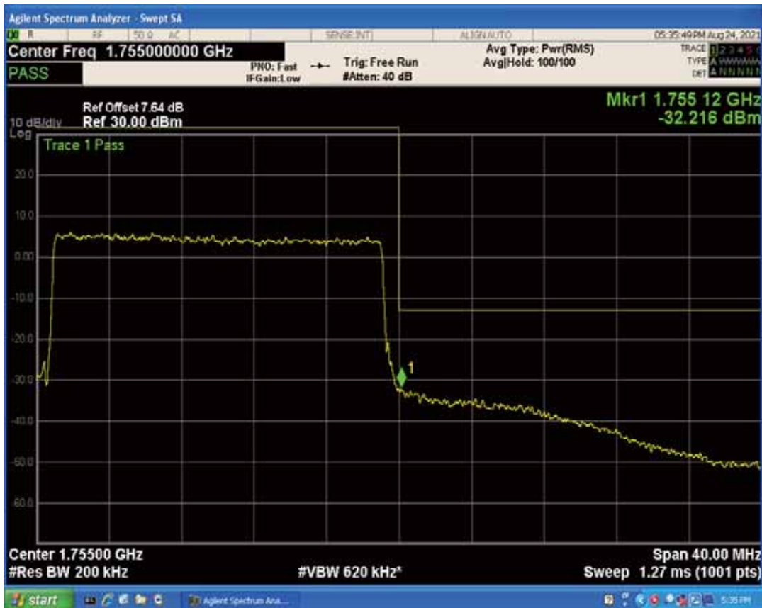
Band4 QAM16 BW=20MHz Channel=20300 RB Size=1 Position=#0
