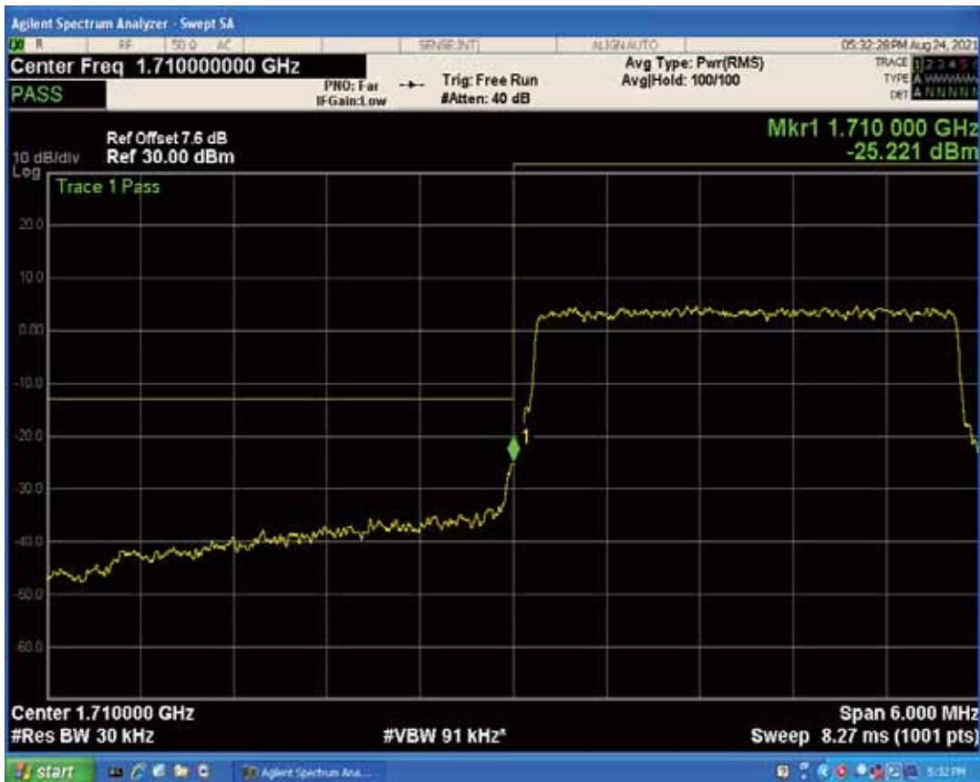
Band4 QPSK BW=3MHz Channel=20385 RB Size=1 Position=#Max
