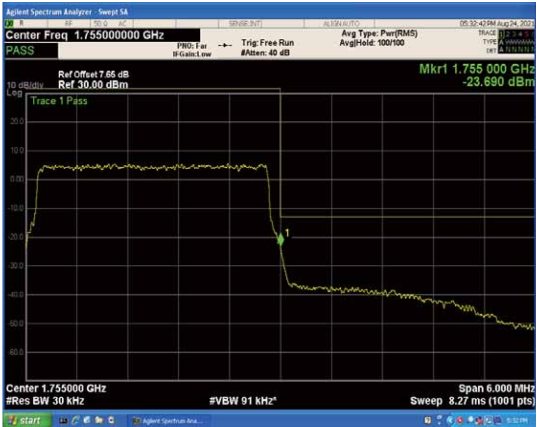
Band4 QAM16 BW=3MHz Channel=20385 RB Size=1 Position=#Max
