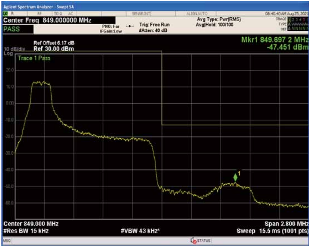
Band5 QAM16 BW=1.4MHz Channel=20643 RB Size=1 Position=#Max
