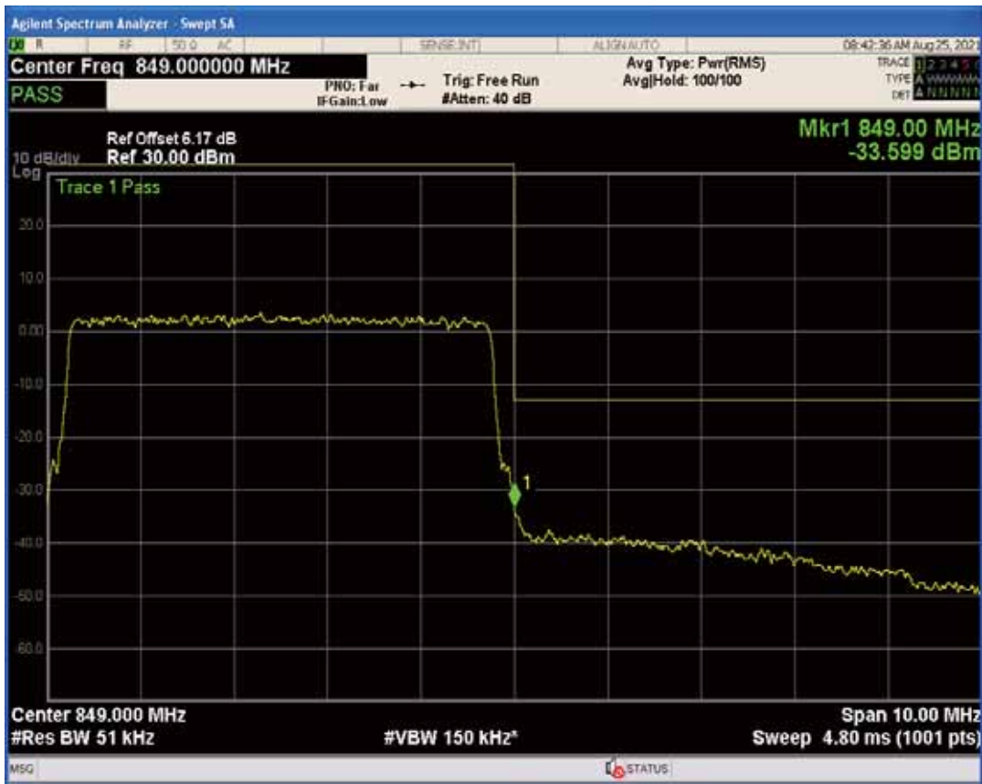
Band5 QAM16 BW=5MHz Channel=20625 RB Size=1 Position=#Max
