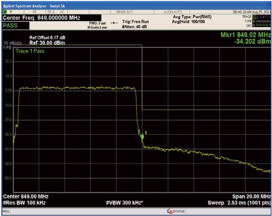
Band7 QPSK BW=5MHz Channel=20775 RB Size=1 Position=#0
