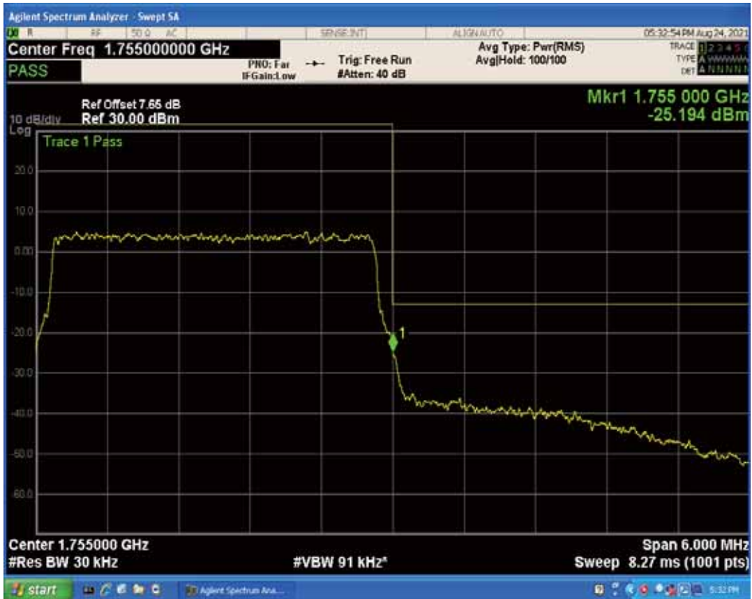
Band4 QPSK BW=5MHz Channel=19975 RB Size=1 Position=#0
