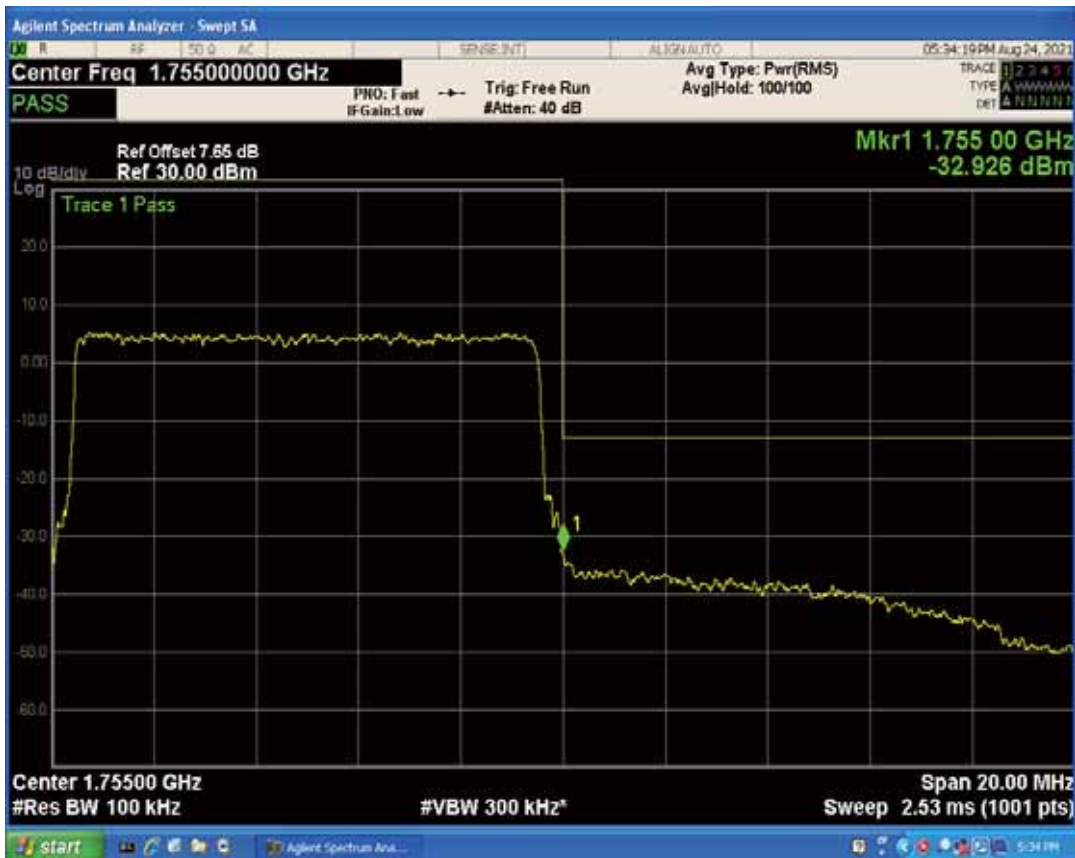
Band4 QAM16 BW=10MHz Channel=20350 RB Size=1 Position=#0
