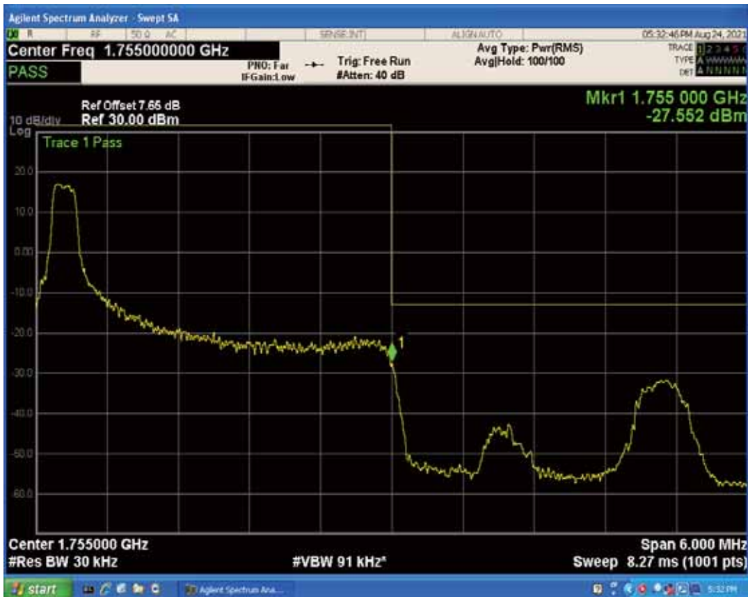
Band4 QPSK BW=3MHz Channel=20385 RB Size=15 Position=#0
