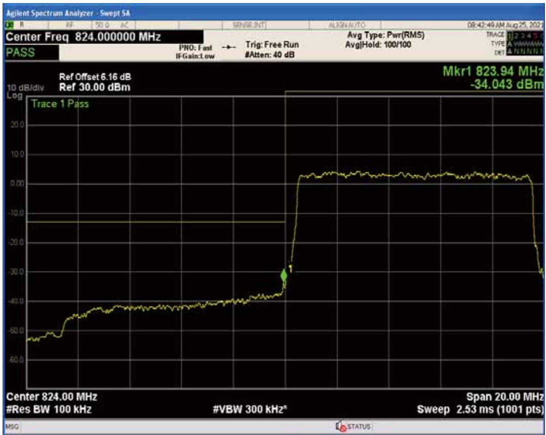
Band5 QAM16 BW=10MHz Channel=20450 RB Size=1 Position=#0
