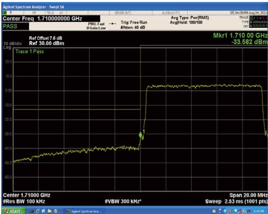
Band4 QPSK BW=10MHz Channel=20350 RB Size=1 Position=#Max
