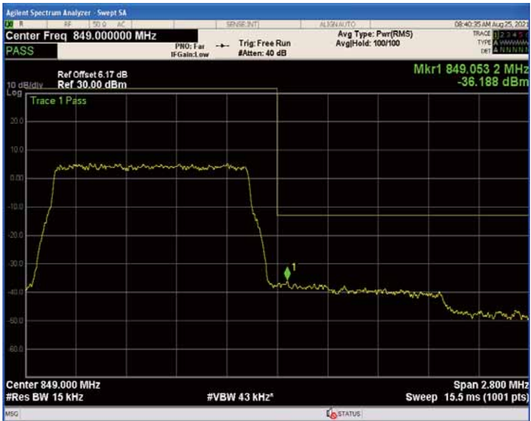
Band5 QAM16 BW=1.4MHz Channel=20643 RB Size=1 Position=#0
