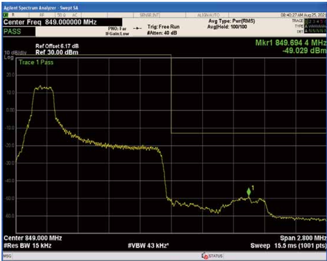
Band5 QPSK BW=1.4MHz Channel=20643 RB Size=1 Position=#Max
