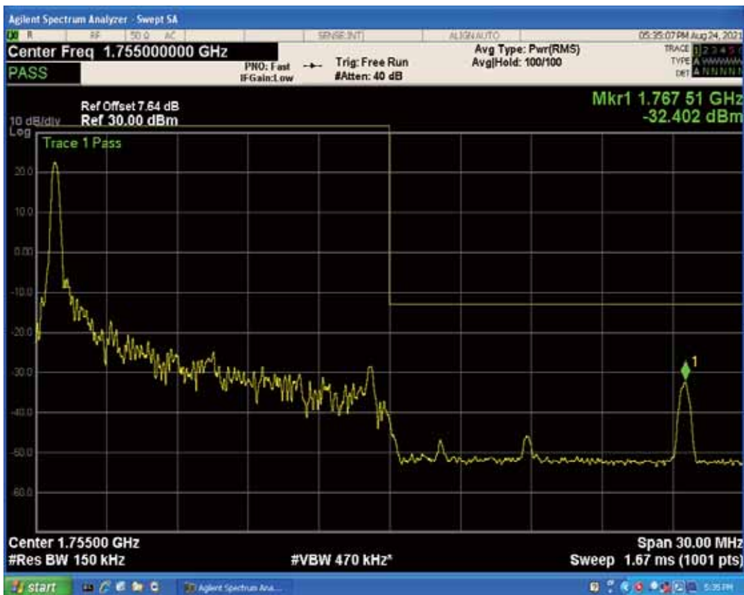
Band4 QPSK BW=15MHz Channel=20325 RB Size=75 Position=#0
