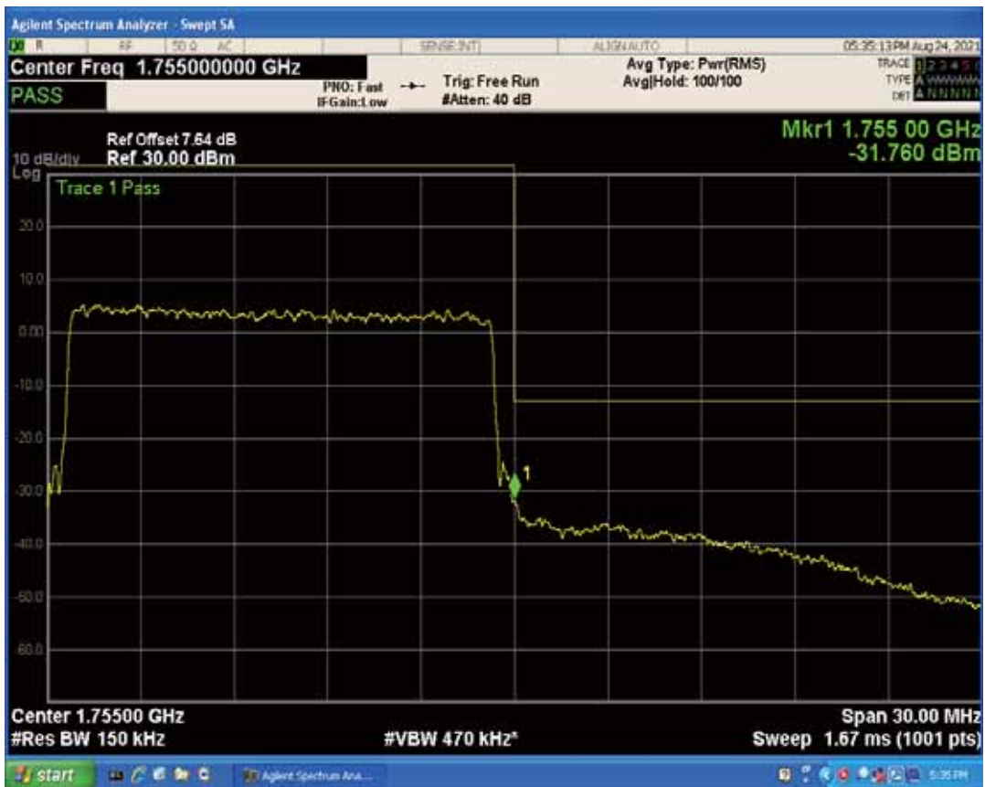
Band4 QPSK BW=20MHz Channel=20050 RB Size=1 Position=#0
