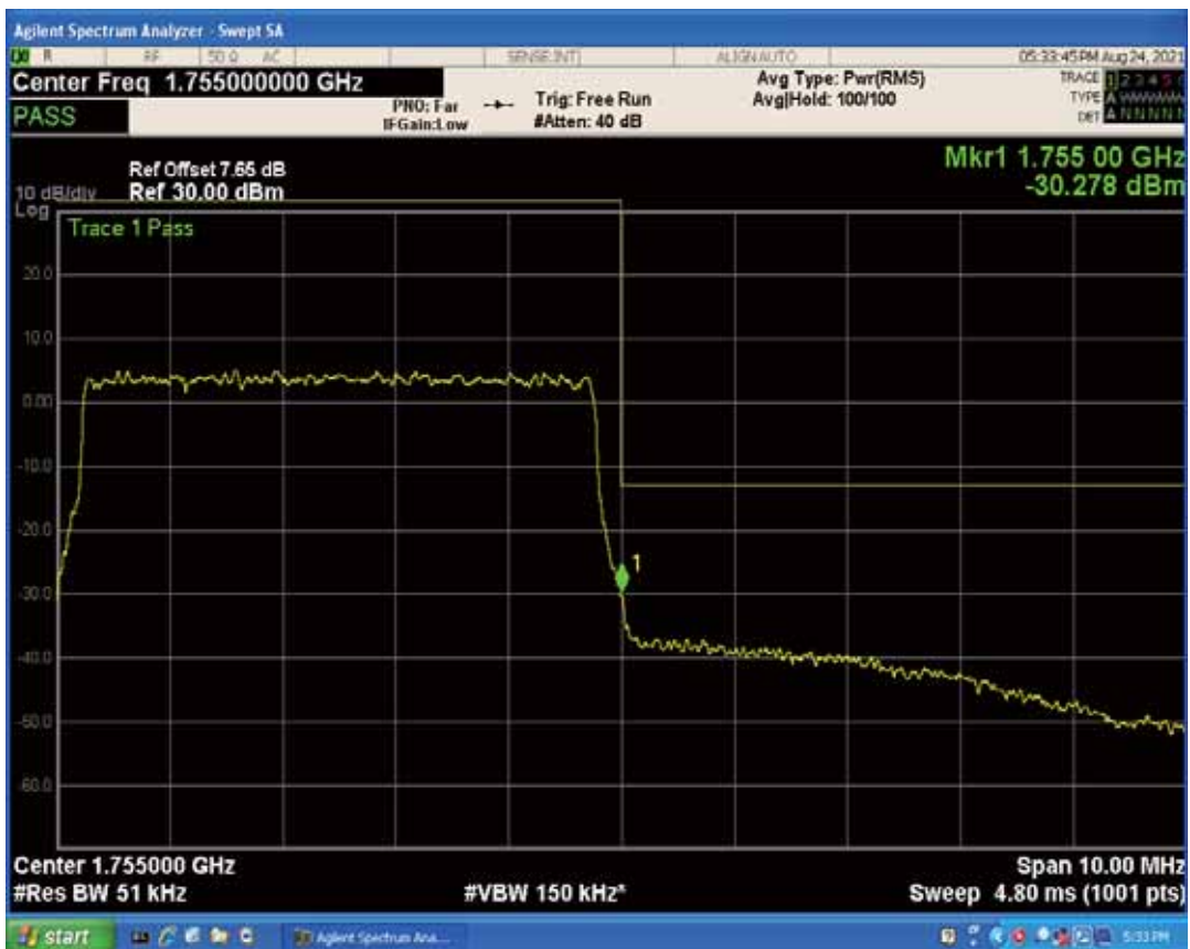
Band4 QPSK BW=10MHz Channel=20000 RB Size=1 Position=#Max
