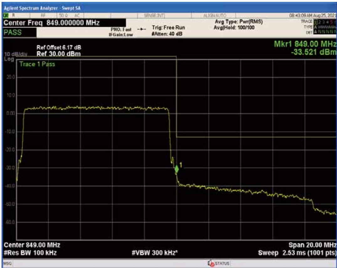
Band5 QAM16 BW=10MHz Channel=20600 RB Size=1 Position=#0
