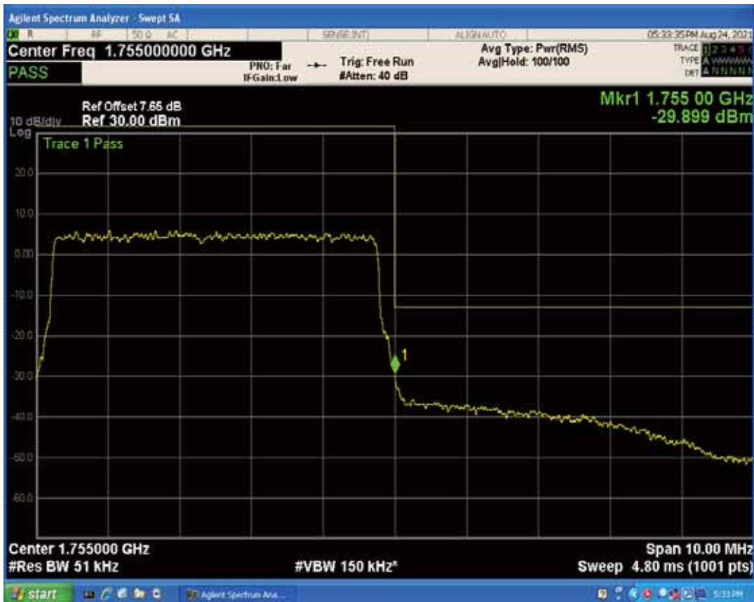
Band4 QAM16 BW=5MHz Channel=20375 RB Size=1 Position=#0
