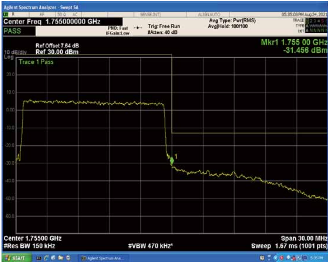
Band4 QAM16 BW=15MHz Channel=20325 RB Size=1 Position=#Max
