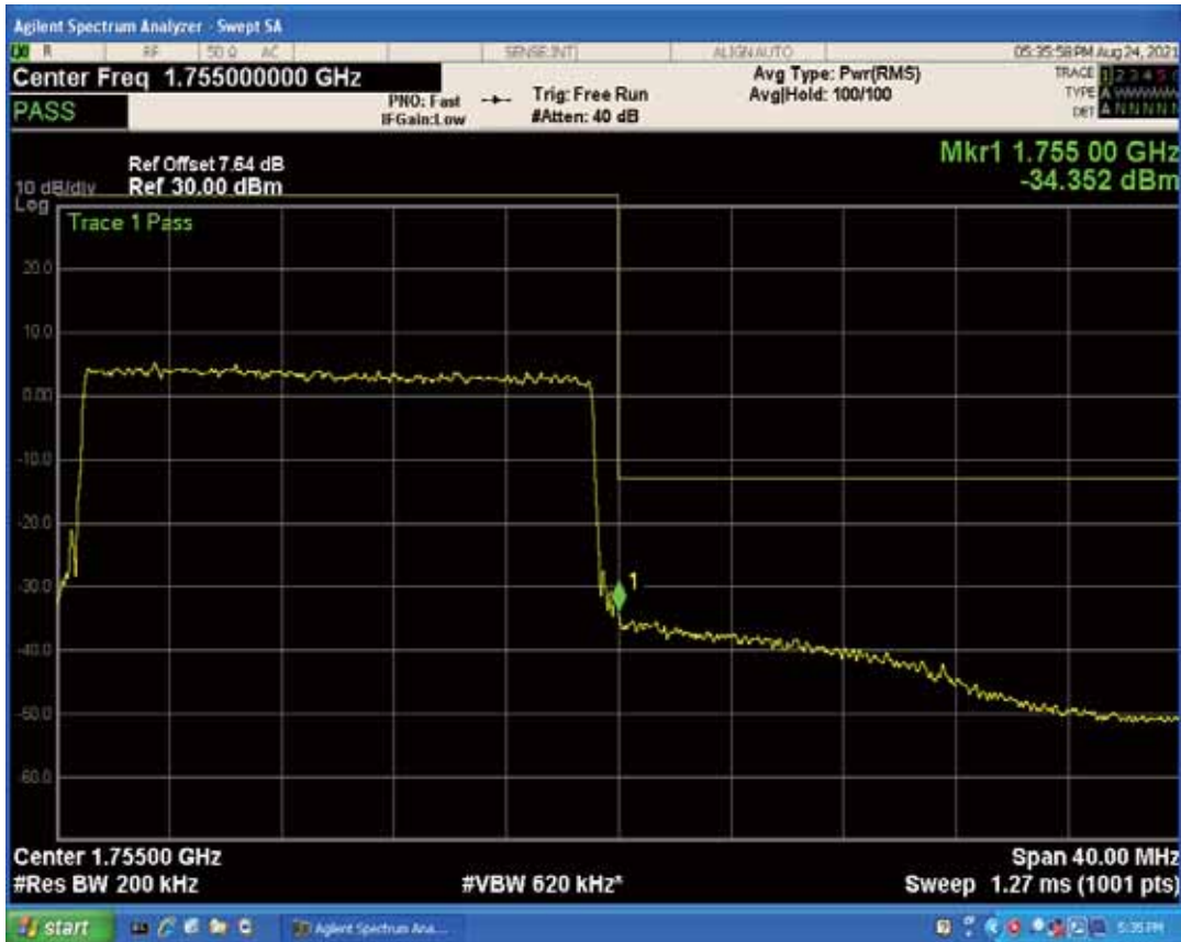
Band5 QPSK BW=1.4MHz Channel=20407 RB Size=1 Position=#0
