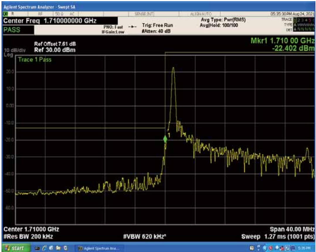
Band4 QAM16 BW=20MHz Channel=20050 RB Size=1 Position=#Max
