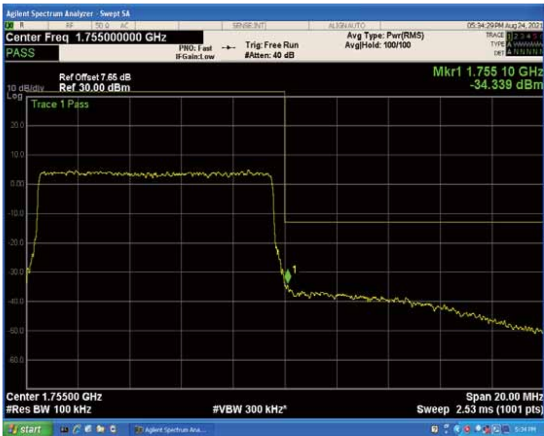
Band4 QPSK BW=15MHz Channel=20025 RB Size=1 Position=#0
