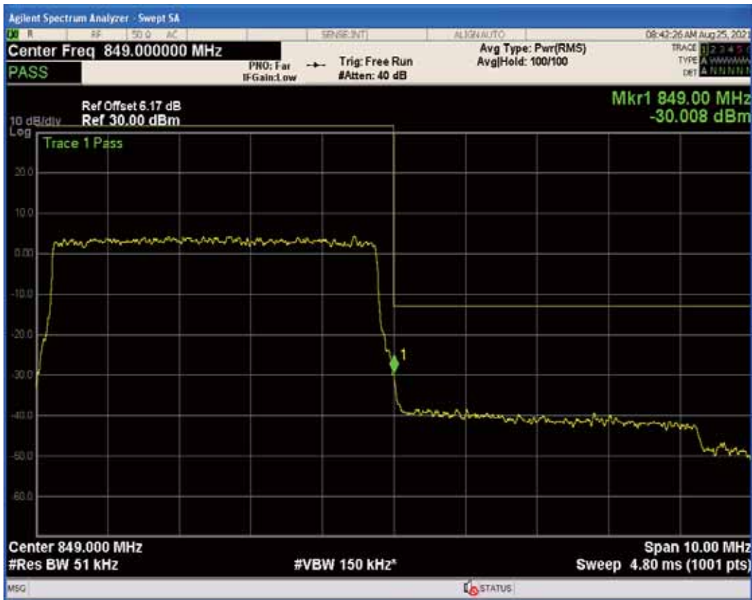
Band5 QAM16 BW=5MHz Channel=20625 RB Size=1 Position=#0
