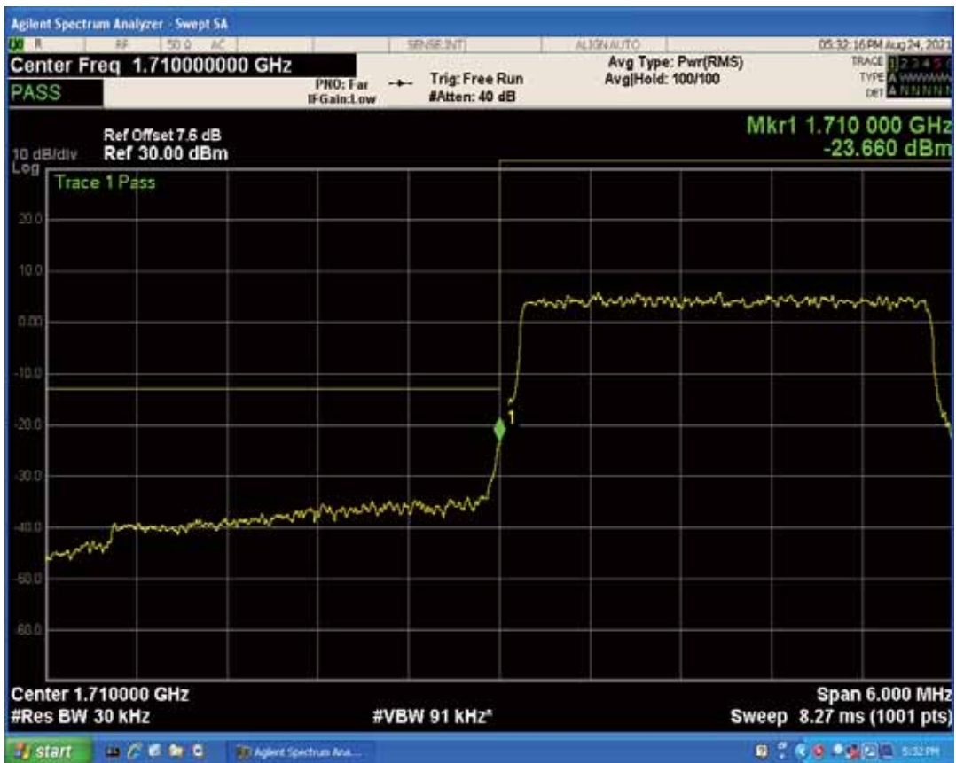
Band4 QAM16 BW=3MHz Channel=19965 RB Size=1 Position=#Max
