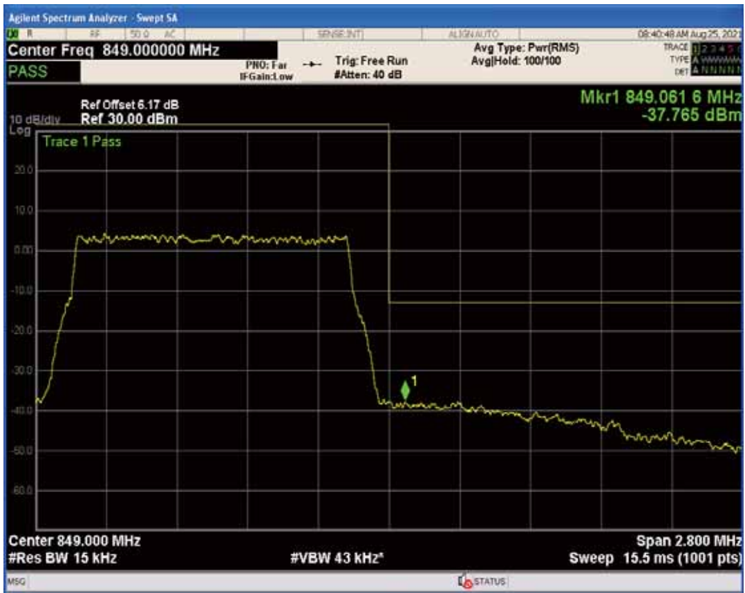
Band5 QPSK BW=3MHz Channel=20415 RB Size=1 Position=#Max
