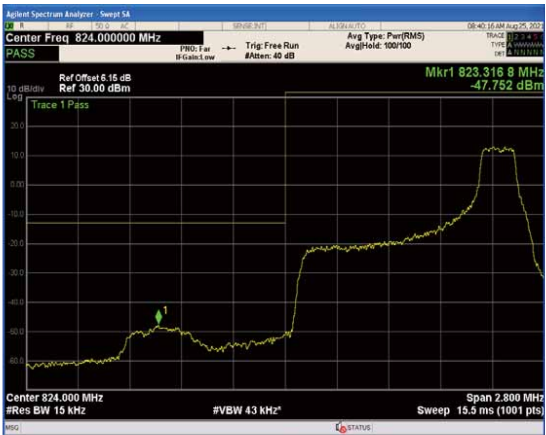
Band5 QAM16 BW=1.4MHz Channel=20407 RB Size=6 Position=#0
