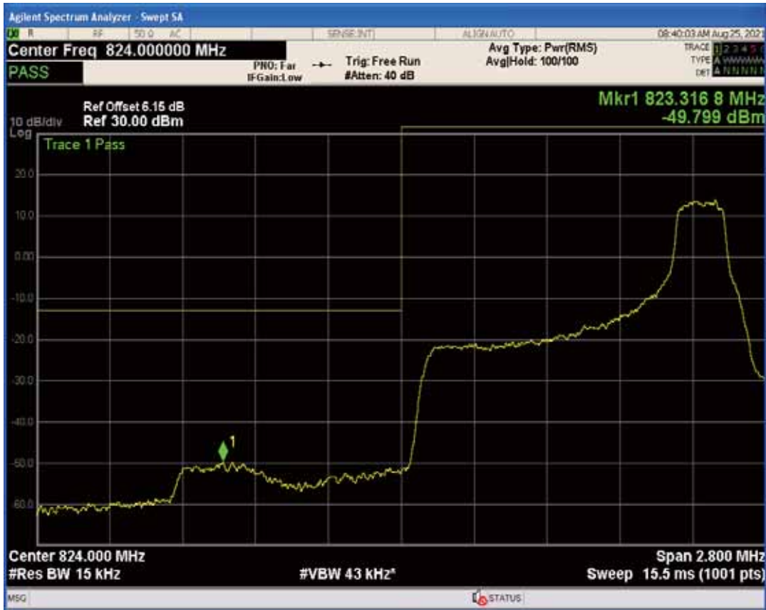
Band5 QPSK BW=1.4MHz Channel=20407 RB Size=6 Position=#0
