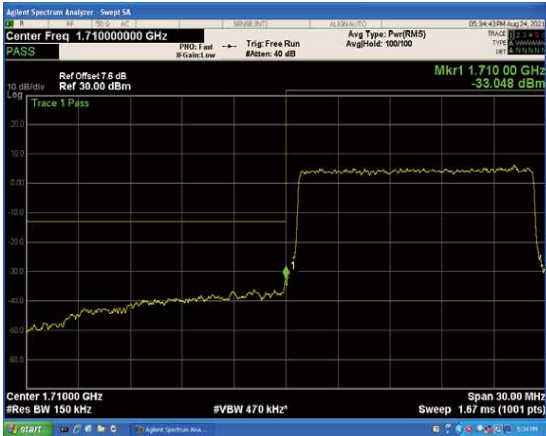
Band4 QAM16 BW=15MHz Channel=20025 RB Size=1 Position=#Max
