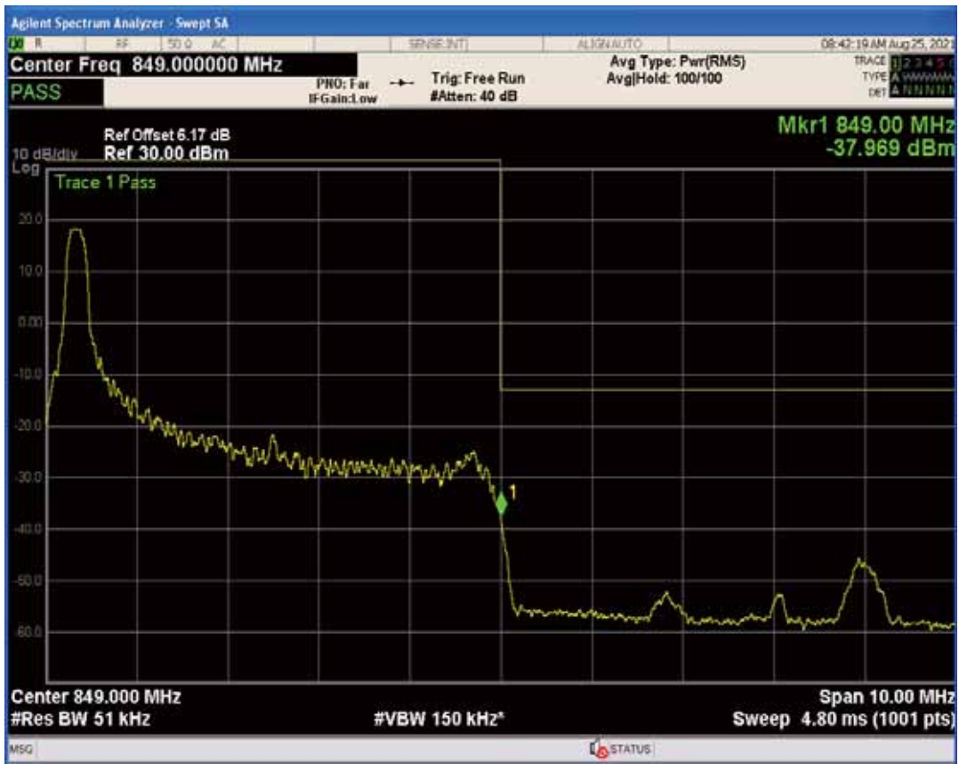
Band5 QPSK BW=5MHz Channel=20625 RB Size=1 Position=#Max
