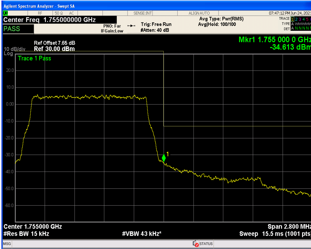
Band4 QAM16 BW=1.4MHz Channel=20393 RB Size=1 Position=#0
