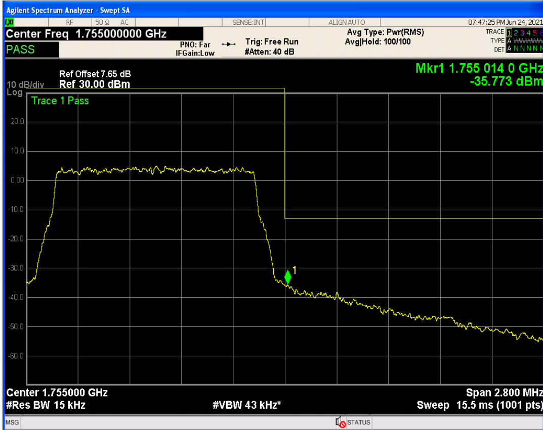
Band4 QPSK BW=3MHz Channel=19965 RB Size=1 Position=#Max
