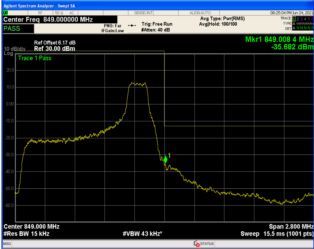
Band5 QPSK BW=1.4MHz Channel=20643 RB Size=6 Position=#0
