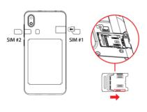
Note: To remove the SIM card, place your finger on the SIM puller and slide it out.
