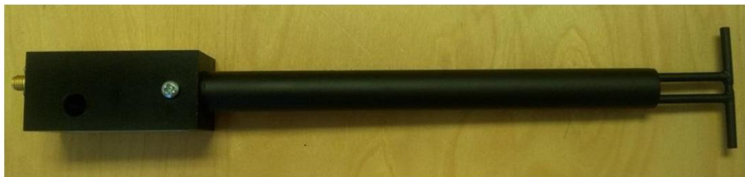
Figure 1 – MVG COMOSAR Validation Dipole
